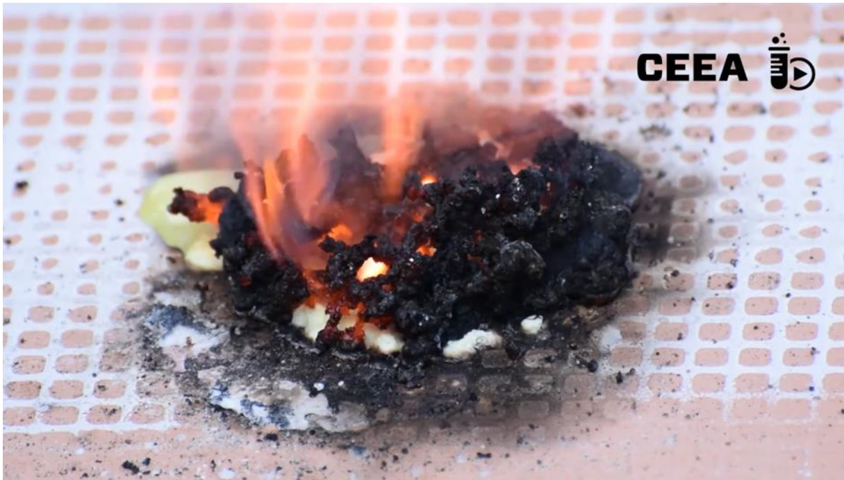
Burning rocket fuel from sugar and potassium nitrate
