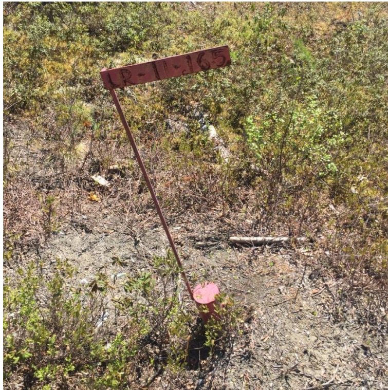
Figure 1: Drill hole casing with casing cap
