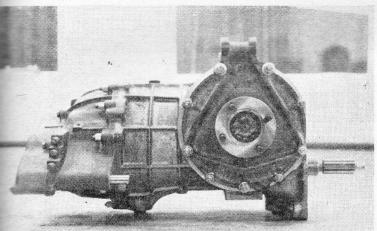
FIVE-SPEED allpurpose gearbox (left). All ratios are changed by removing the rear section of the unit in situ. Any selection of ratios can be fitted in half an hour.
