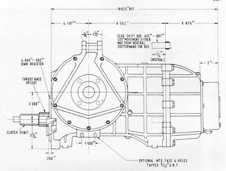
SIDE VIEW of the gearbox (above), showing the varinstallation dimensions. Note the overall length is only 18.6 ins.
