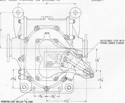
REAR VIEW of the gearbox, showing the adjustable stop with spring-loaded plunger.
