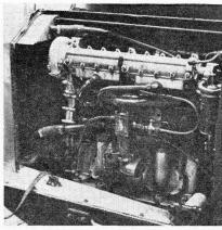
FOUR-CYLINDER engine, of 3,295 c.c., develops 100 b.h.p. at 3,200 r.p.m.
