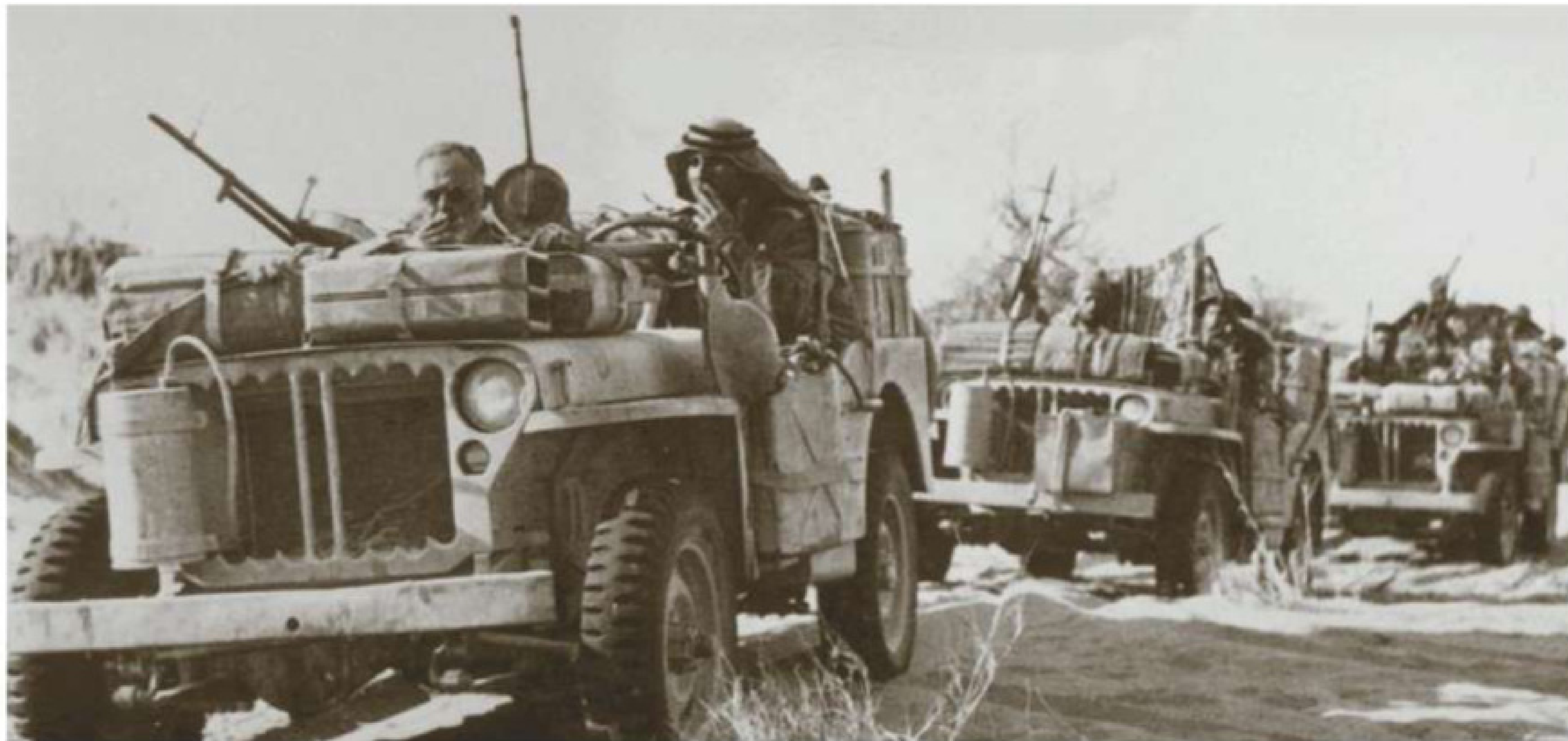
Condenser tanks and radiator grilles hacked to boost air flow are hallmarks of jeeps run by British irregulars. These Special Air Service men are embarking on a raid.
