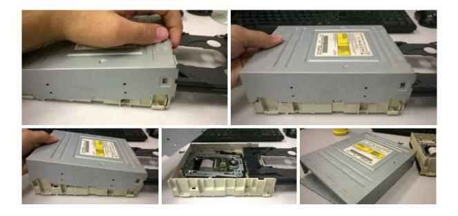
Now on the sides of the press the marked parts on the images and pull the front of the driver, after that finish taking off the metal cover.
