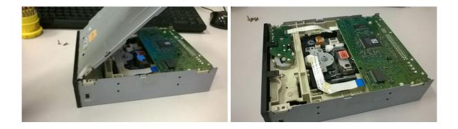
The first thing to do is to loose the four screws under the driver, after that you can pull the cover.
