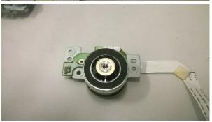
The motor used to spin the CD or DVD is a brushless motor, that means that you can't simply connect two wires in a battery an it will spin, for that, you will need a Electronic Speed Controller (ESC) and maybe some mods, following are some instructables with motors like this.
