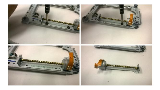
The motor used to movement the laser is a stepper motor, stepper motors are very good to positioning, the signal sent to the motor makes it move to a determined position.
