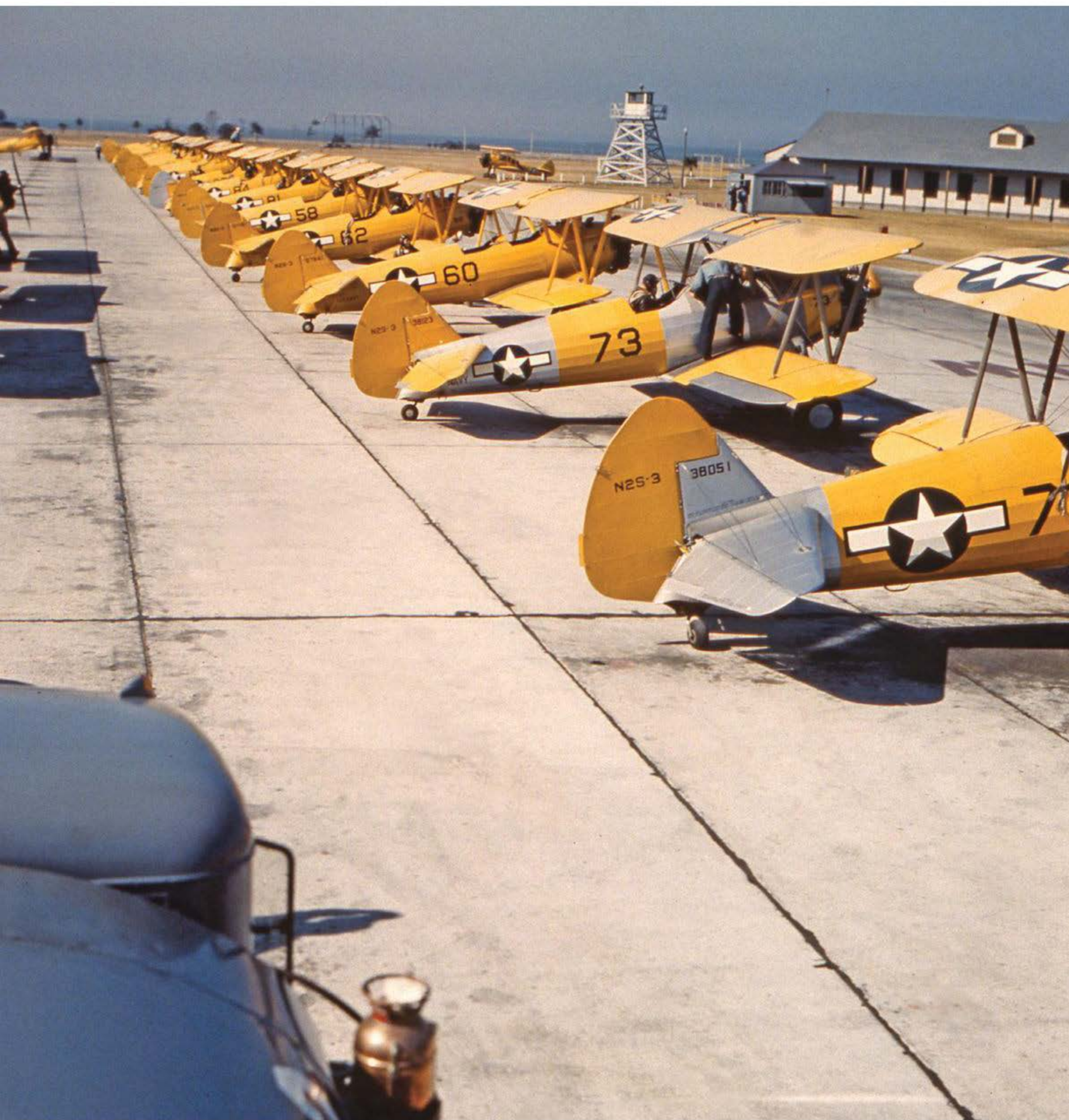
At the beginning of the war, the Navy used the N3N and the Army used half a dozen different trainers. Partway through the war, both services began to standardize on the Model 75 Boeing/Stearman Kaydet. In the Army, it was designated the PT-17 (or some minor variant thereof); in the Navy, it was the N2S. (Photo courtesy of Stan Piet)
