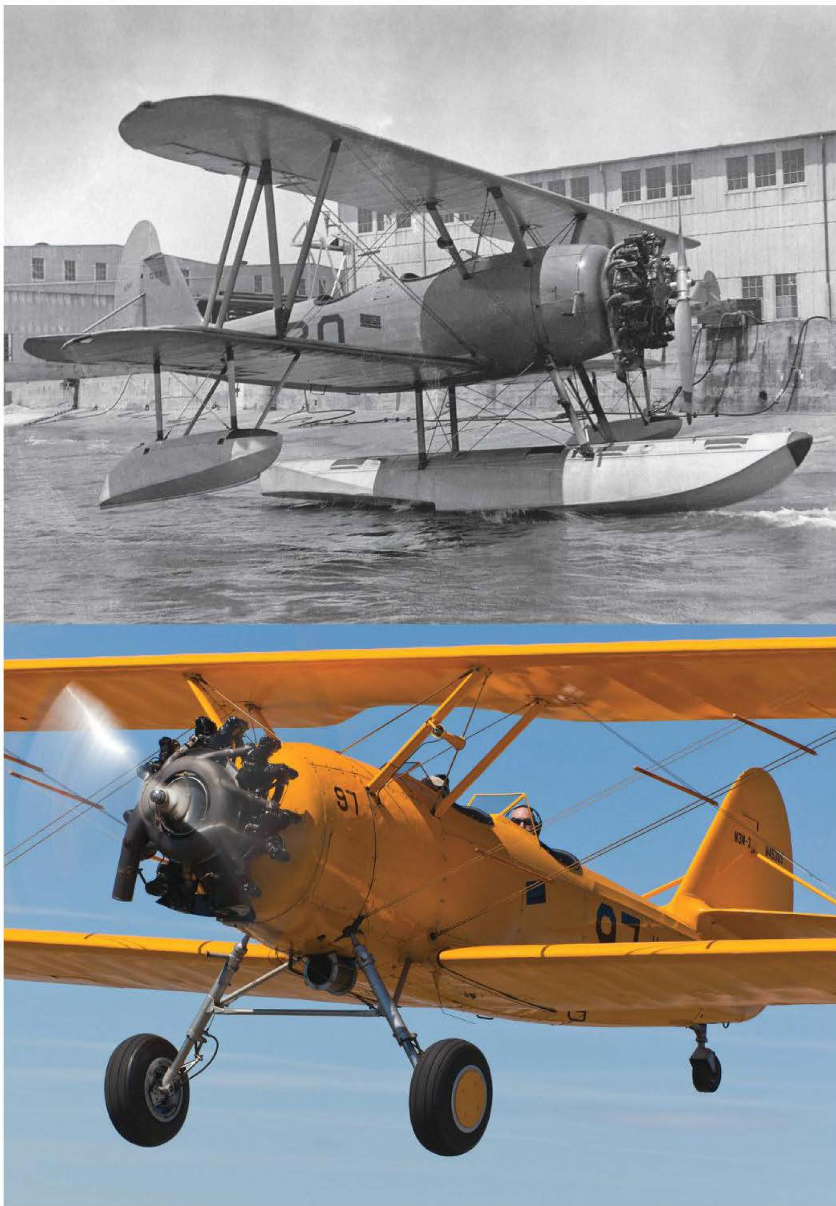
In 1935, the Navy decided that it needed an airplane that it felt fit its training purposes better than the Stearman, so it designed and built the N3N in its own facility. Eventually, the Navy even bought the rights to the R-670 Wright engine and began building its own engines. The design is unique in that, rather than being welded tubes, the fuselage is a triangulated structure using extruded aluminum angles that are bolted together. (Top photo courtesy of Jack Cook; bottom photo by Jim Raeder)
