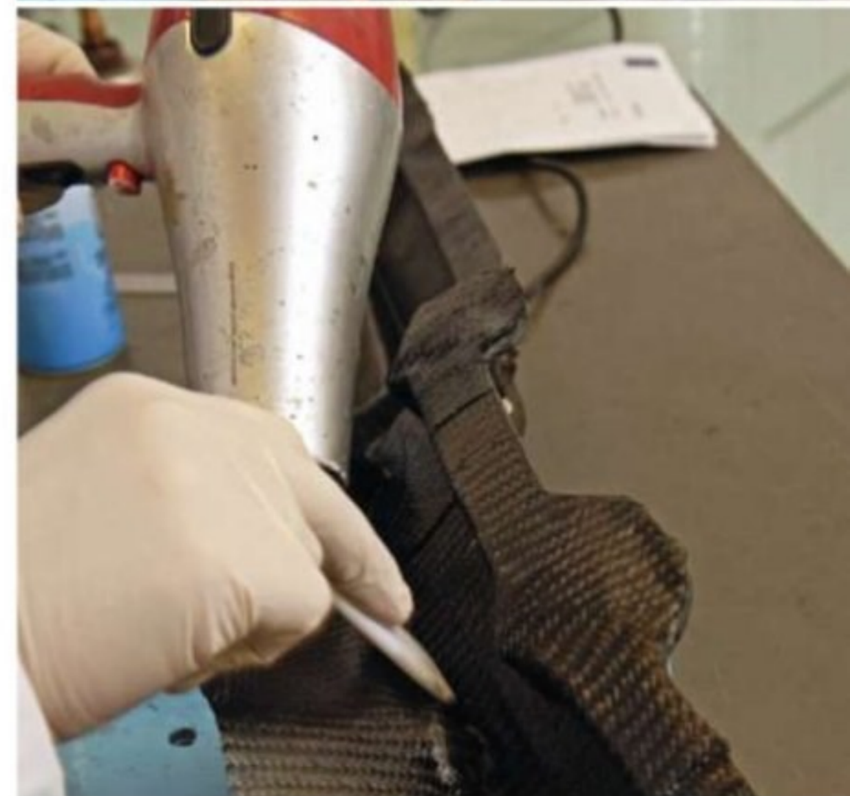
▲ Making a front wing Small pieces of carbon fibre are cut from a roll and stuck into place on moulds to create front and back 'skins'. Once the two skins have been cured in the autoclave at high temperatures, they can be bonded together to form the lightweight and ultra-resilient wing
