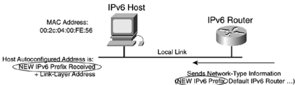
Figure 1-11. A New Unicast IPv6 Prefix Is Advertised on the Local Link During Renumbering
