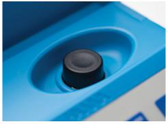
An affixed, light-blocking cover panel closes over the sample cell, reducing stray light from affecting any measurement readings.
