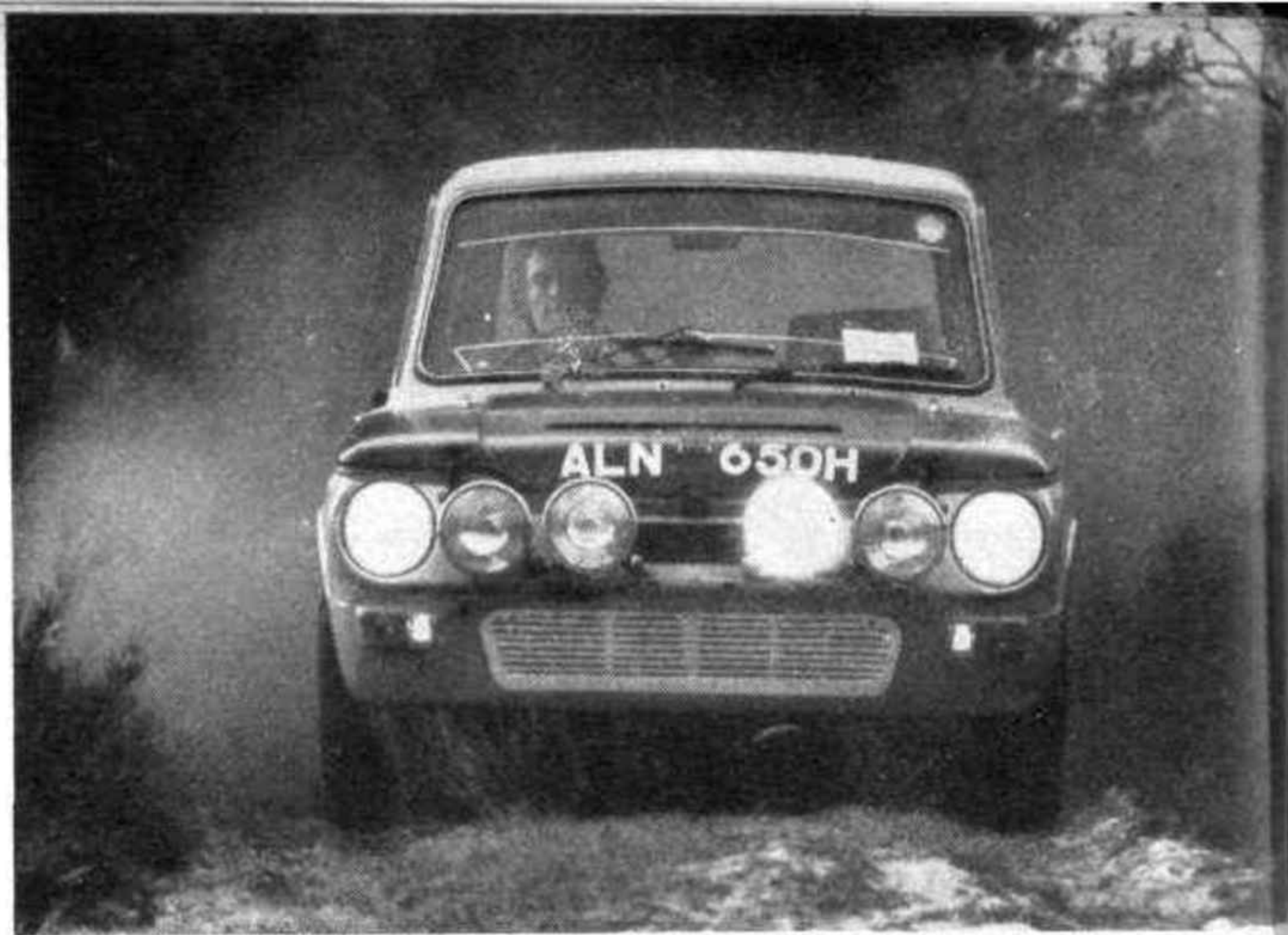
The Special Imp's auxiliary lamps give an ideal spread of light; other electrical equipment includes a heated windscreen. Note the bonnet securing strap and rubber toggles (which are easily forgotten), and the towing hitch attached to one of the front suspension's swinging arms.
