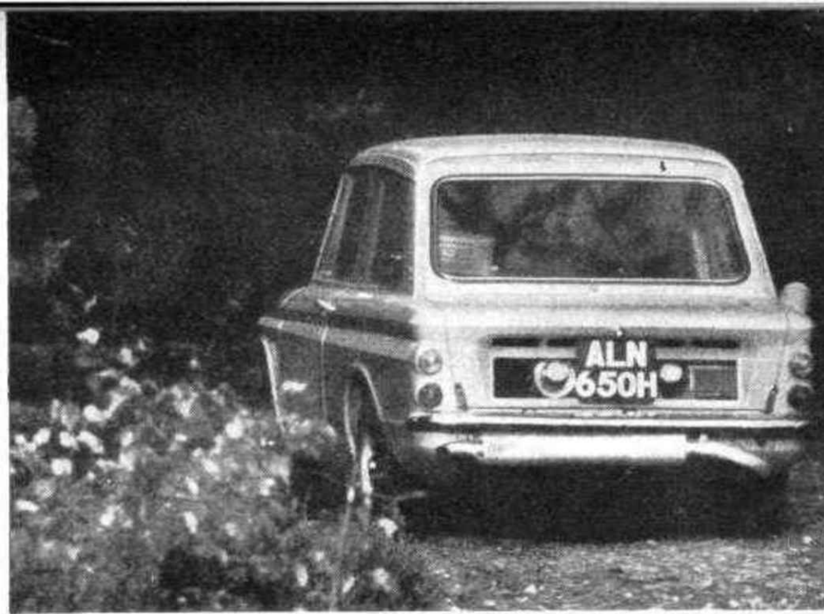
The transversely-located silencer effectively increases ground clearance, but transmits some vibration and noise to the interior: the scoop on the off-side rear wing supplies cold air to the oil-cooler. Small reversing lights on each side of the number-plate emit a surprising amount of light.
