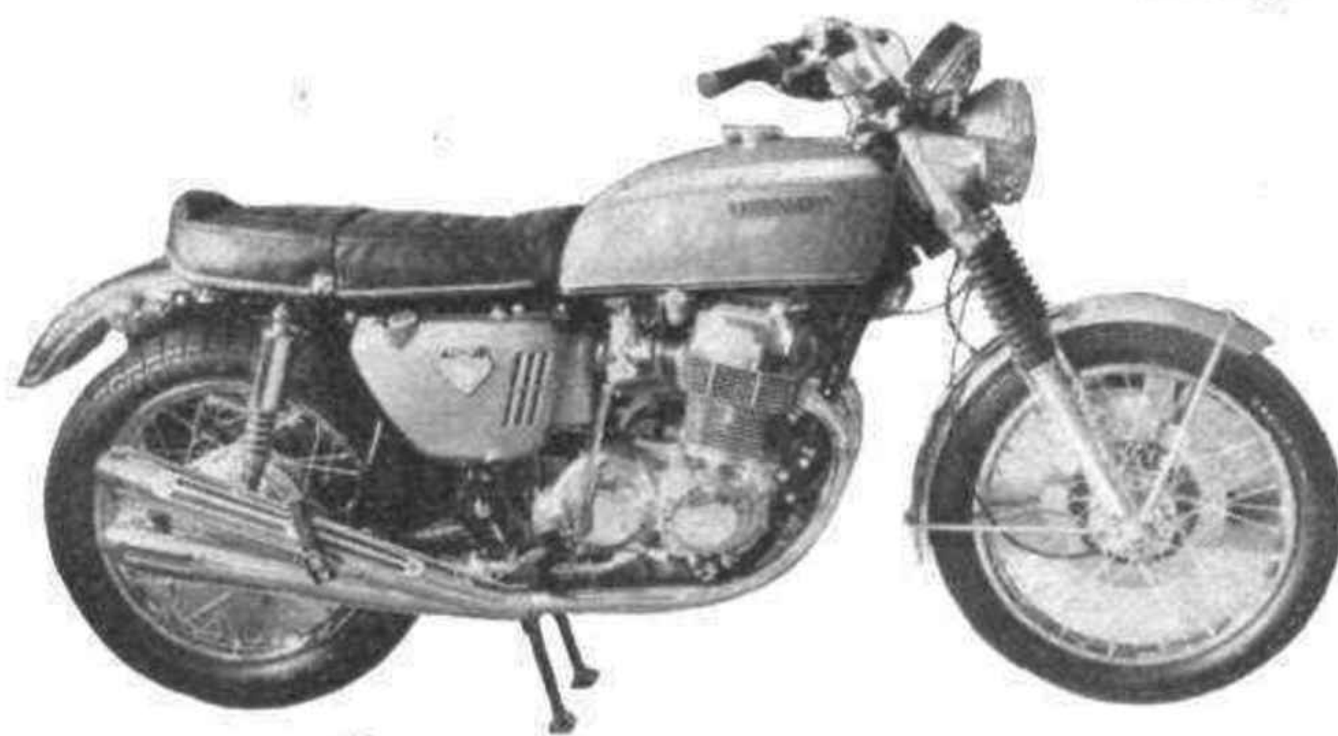
MOST EXOTIC.—The 750-c.c. Honda four-cylinder motorcycle, with twin overhead camshaft air-cooled engine mounted transversely. The whole machine exudes an air of power and intrigue, from its disc front brake to its four megaphone exhausts.
