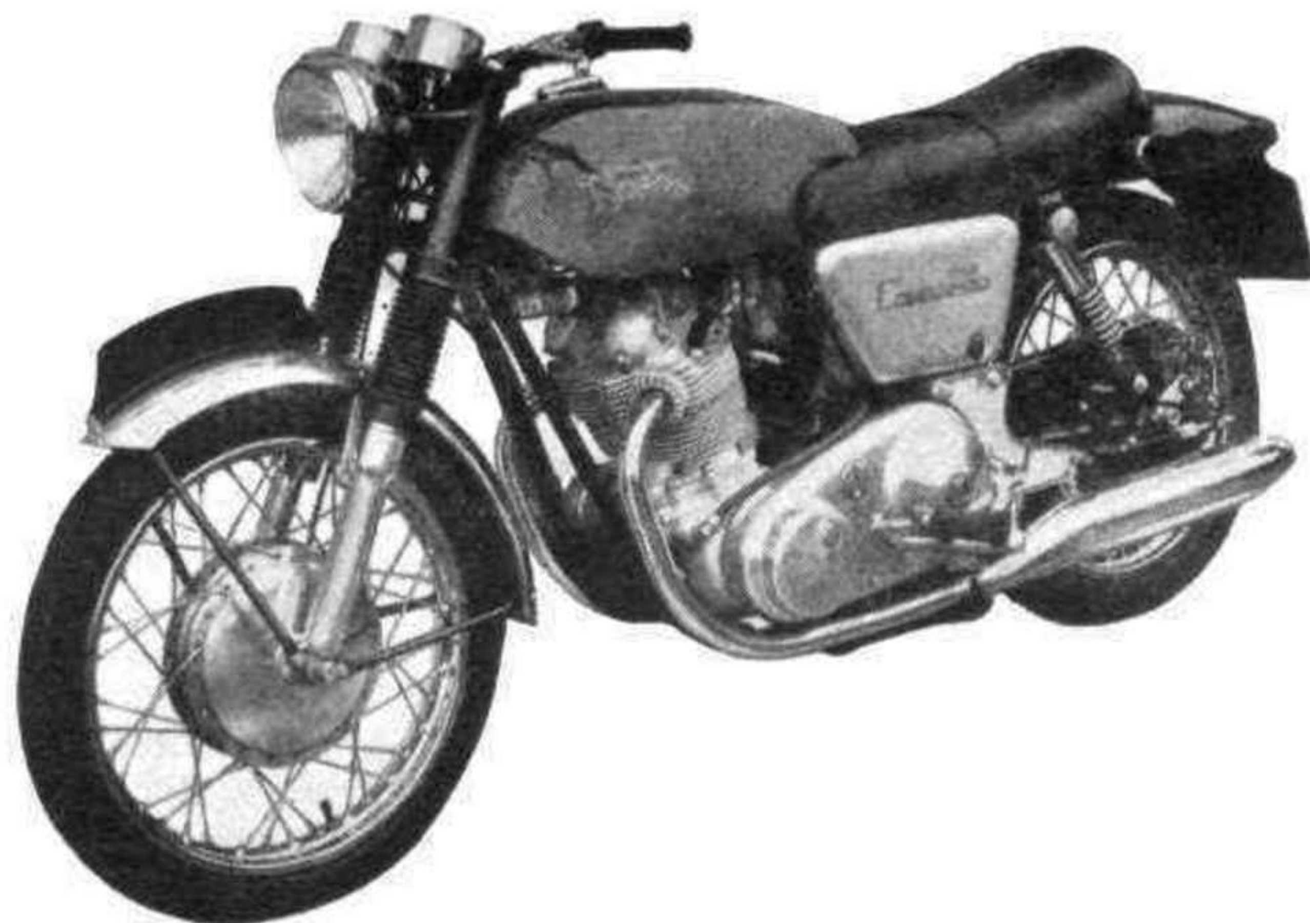
MOST PRACTICAL.—The 750-c.c. Norton Commando is considered to be the best all-rounder in the fast motorcycle world. Although its vertical twin engine is dated, a lot of the roughness inherent in this layout has been eliminated by mounting the engine/gearbox aggregate and rear suspension, on rubber.
