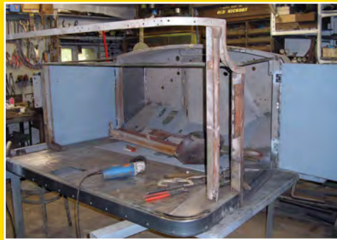
Above: The cab in particular was infested with tin worm. Above right: Most of the cab was replaced. Note that the upright nearest the camera has been completely eaten away at the base.
