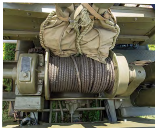
A Garwood winch sits behind the cab and is chain-driven via a power take-off from the transfer case.
