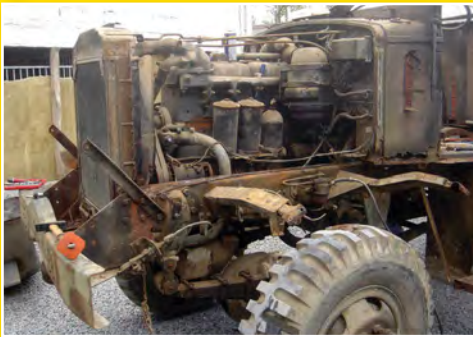
Above: The cab in particular was infested with tin worm. Above right: Most of the cab was replaced. Note that the upright nearest the camera has been completely eaten away at the base.
