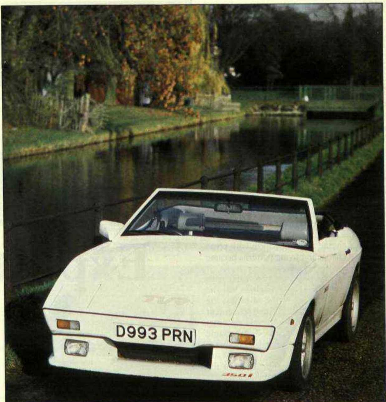
Separate bumper/spoiler mouldings have allowed TVR to ring the changes on a basic shell.
