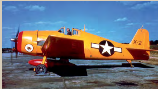
Colour schemes varied on target drone F6F-5Ks. A large number of Hellcats were turned into radio-controlled drones from 1950 to 1957. TAILHOOK ASSOCIATION
