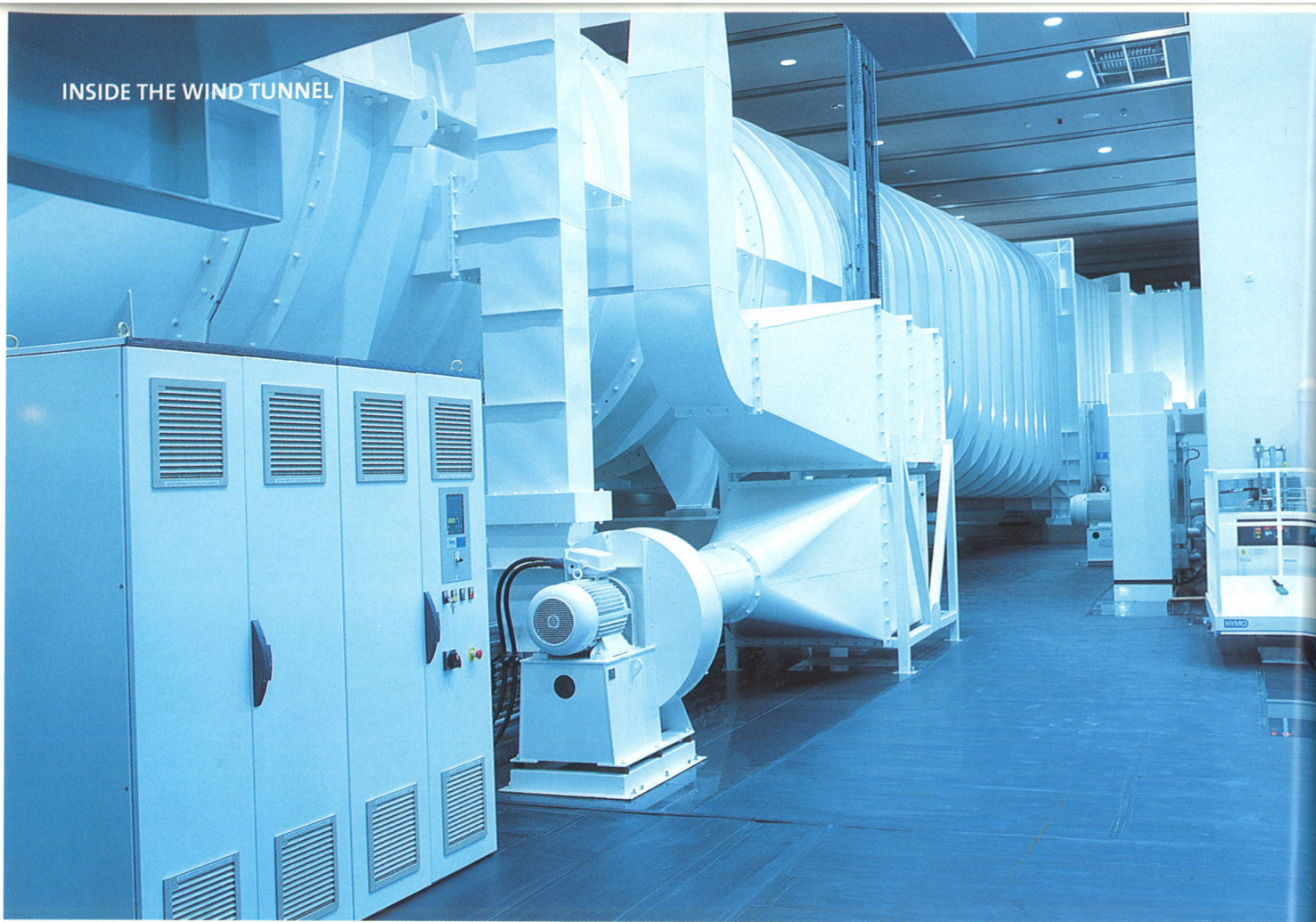
ABOVE The 145-metre long wind tunnel contains 400 tonnes of steel, but such a large structure is entirely necessary to ensure that the airflows produced are as controllable and accurate as possible
