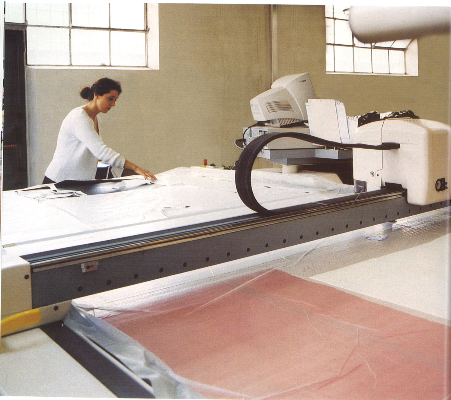
ABOVE The cloth is cut by machine. Up until recently, this process was done by hand, but even this is now computerised – such is the accuracy of the equipment and the need for each and every pair of overalls to be as comfortable and as perfect a fit as the last
