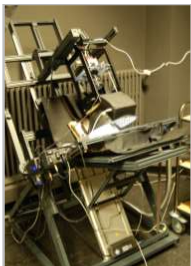
Afb. 8. Conservation Copy Stand en portable lightdome. Afb. 9. Traveller's Conservation Copy Stand.
