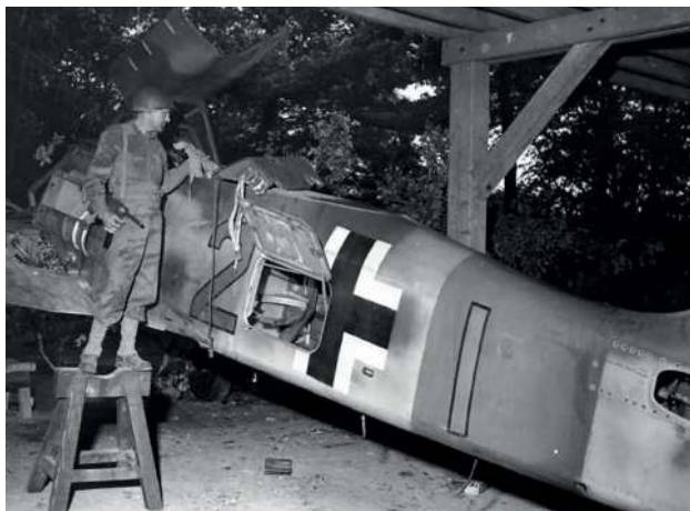
■ Although taken at the end of the war, this photograph shows the small fuselage hatch on the Focke Wulf 190 into which hapless groundcrew members were crammed as units moved up nearer to the invasion area.
