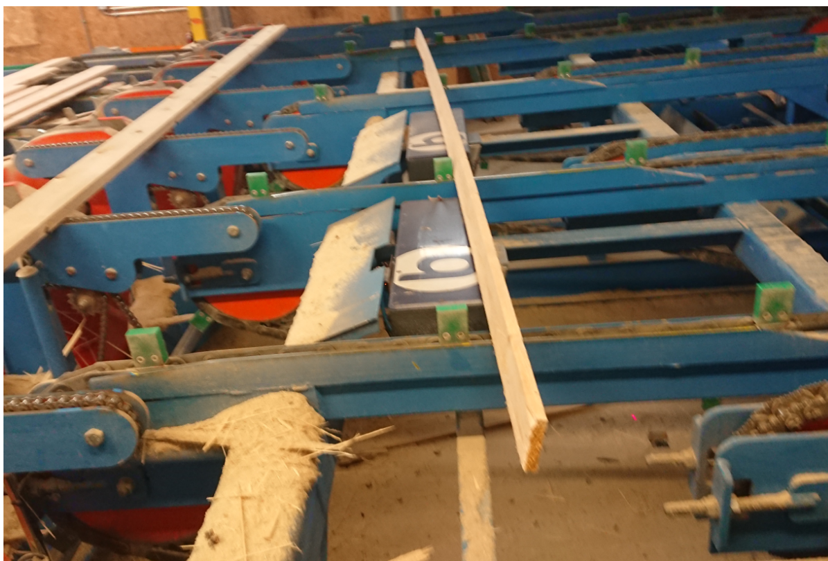
Figure 9. Correct position of timbers on the packing machine. (courtesy of Hekotek)
