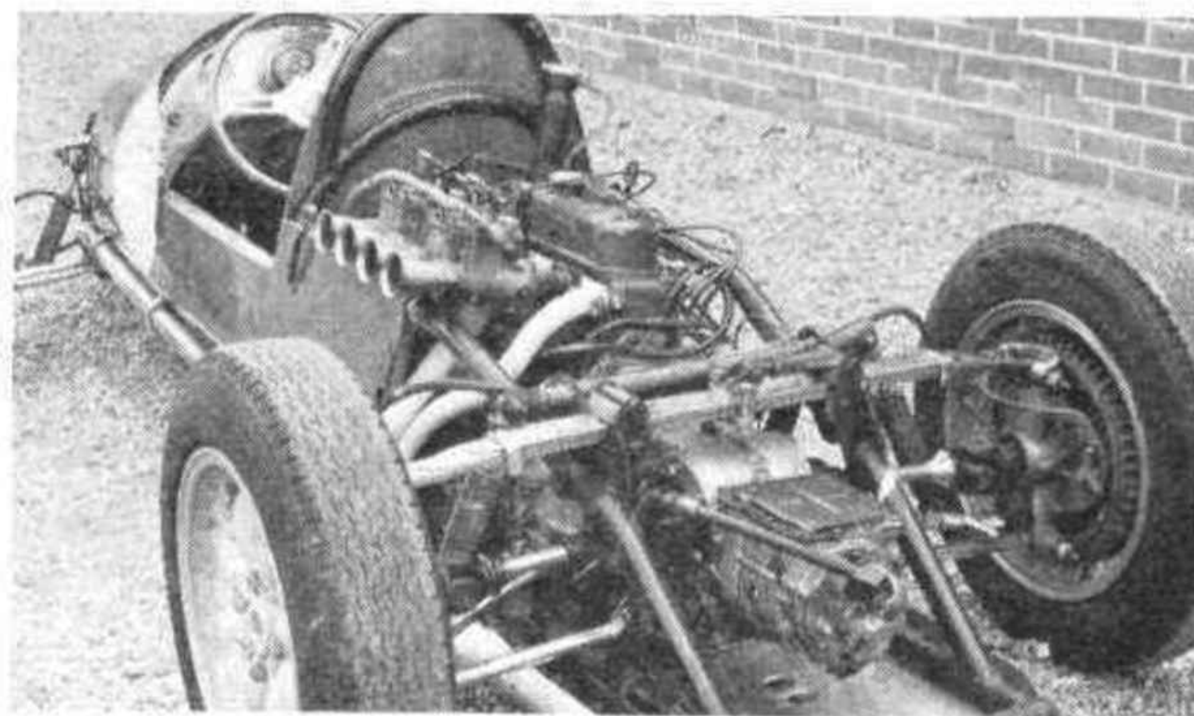
THE WORKS.—The B.M.C. "A" series engine of the Venom with twin Webbers, mated to a Dauphine-Gordini gearbox.
