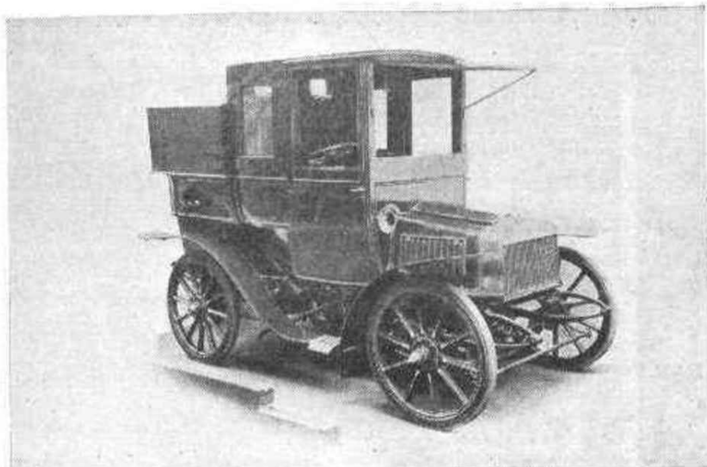
The first Craig-Dörwald, a 2-cylinder 16-h.p. traveller's car, supplied at the request of a client in 1903.
