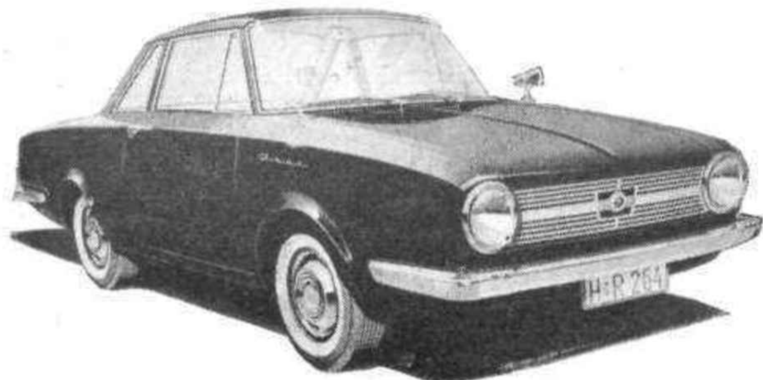
AN ARTIST'S impression of the new Goggomobil coupé, fitted with a 993-c.c. 4-cylinder overhead camshaft engine.
