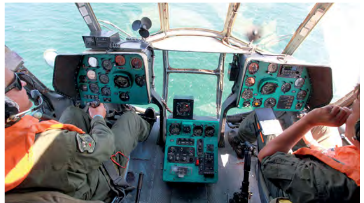
Below: The Cold War-era Mi-17 cockpit remains little changed, although civilian-standard GPS receivers and VOR/ILS/DME equipment have been added.
