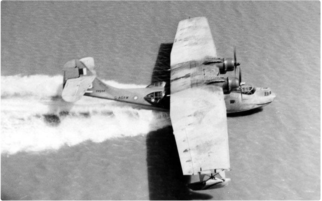
ABOVE Catalina G-AGFM Altair Star rises on to the step during take-off from Koggala Lake. The RAF's Catalina IBs, powered by a pair of Pratt & Whitney R-1830-92 Twin Wasp air-cooled radial engines, were supplied against Lend-Lease requisitions, as were the two IVAs and sole IVB also used on Qantas's wartime Indian Ocean service.
