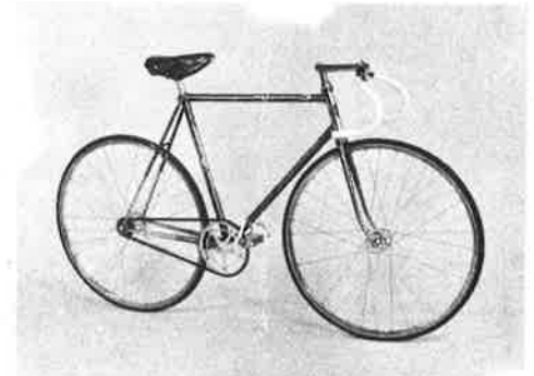
570 PROFESSIONAL SUPER PISTA - 531 Reynold Tubing - All Campagnolo - 1/2 pitch, Dunlop tubulars - nylon seat. Sizes : 21", 22", 23", 24" colors: in Red & Blue.
