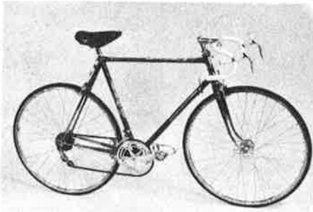
585 PROFESSIONAL TOUR DE FRANCE - All 531 Reynolds tubing double butted - stronglight Super Competition cotterless crank set 52 X 44 - Lyotard pedals- huret derailleurs Prestige group, Huret fork ends - Mafac Racer brakes - Dural handlebars & stem - Mavic rims - Atom quick release HF hubs- Tubulars - Nylon saddle - Atom freewheel 14 to 26. Sizes : 21" 22" 23" 24" 25" Colors: White, Aquamarine blue (vert omnium), red.
