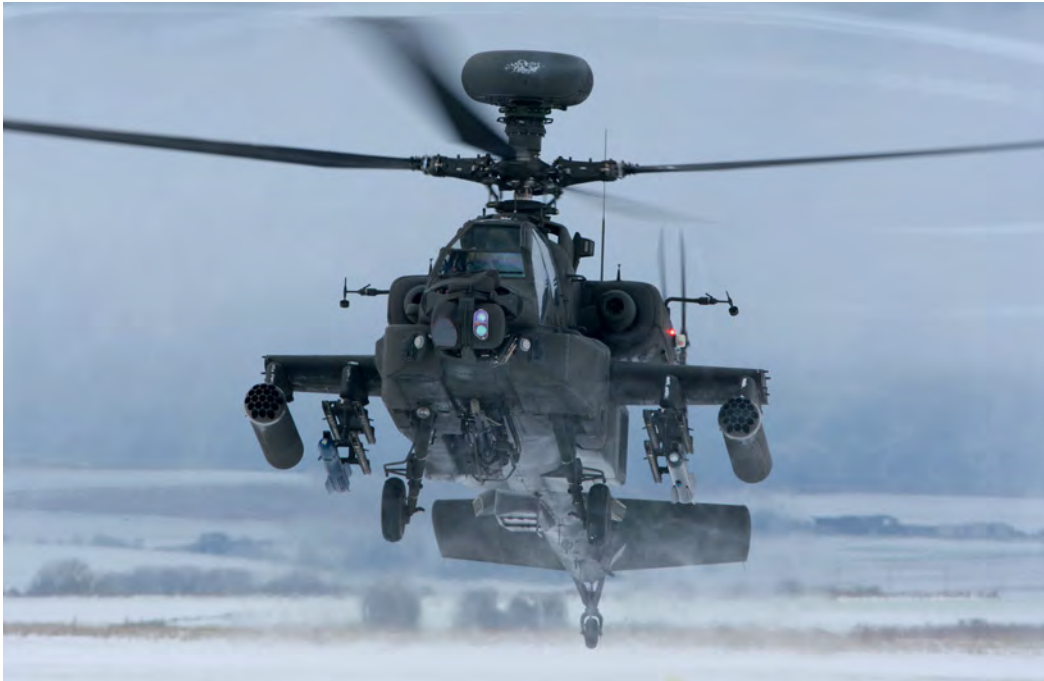
Above: Wattisham-based Apache AH1 callsign 'Gunship 54' conducts whiteout snow landings on Netheravon Airfield, Wiltshire, during a Mission Rehearsal Exercise in February 2009. Whiteouts are similar in terms of visibility and type of approach to brownout conditions in the hot and sandy climate of Afghanistan, except that sand is a lot more abrasive on aircraft components, especially the rotor blades. Rich Pittman
