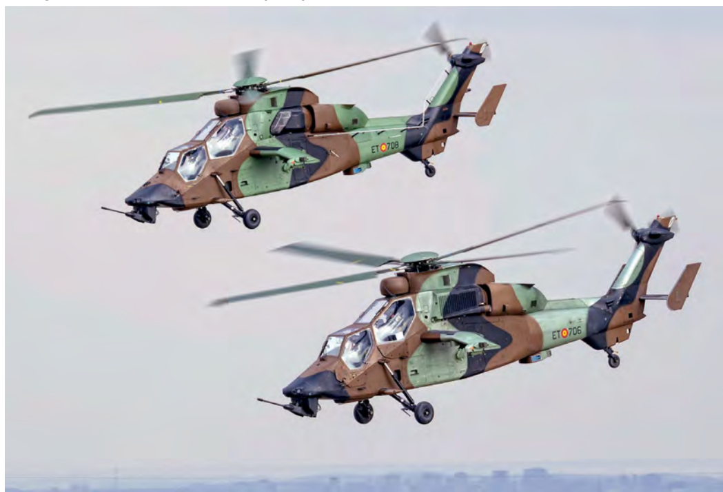
Below: BHELA I based at Almagro operates the Tigres, which are replacing the last few Bo105s. A Tigre HAP (nearest) is escorted by a Tigre HAD after taking off from Colmenar Viejo air base. The major external difference is the engine housing, as the HAD has a newer MTR390-E powerplant. Roberto Yáñez
