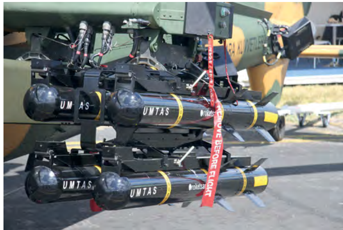
Above: The UMTAS long-range anti-tank missile is one of the T129's main weapons. Alan Warnes
