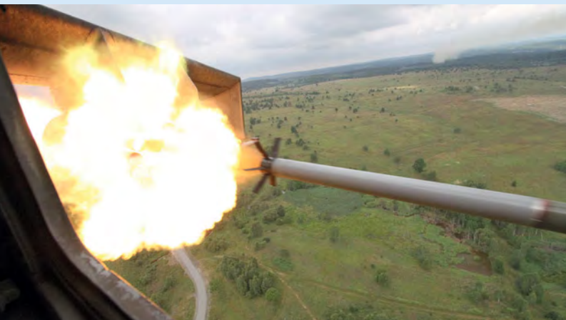
An S-8 is unleashed from its B-8V20 pod. The S-8 is the helicopter's primary unguided rocket and replaced the less reliable and smaller S-5. Jaroslav Špaček
