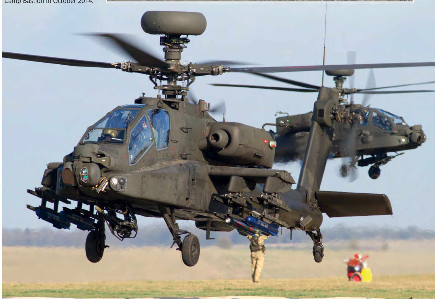
Above: An Apache AH1 prepares to lift off from a forward refuelling point during an exercise on Salisbury Plain. Note the black Hellfire Collective Training Missile (CTM) fitted on the port side of the Apache. The CTM pod can simulate targets for engagement as well as hits to the aircraft itself, and can communicate with other aircraft carrying the pod. It's often used in conjunction with a blue M34 Hellfire training round. Chris Lofting
