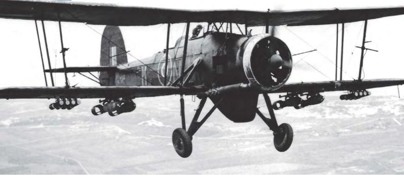
ABOVE: Armed with a variety of bombs and flares and showing the ASV radar radome between the undercarriage. the antiquated appearance of the Swordfish III - this is NF374 belied the type's effectiveness for night inshore patrols. VIA NORMAN WILLIAMSON
