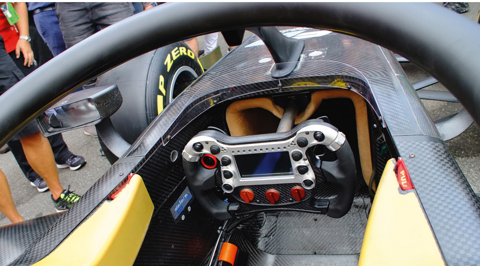
Above: The cockpit features extra Zylon panels which has had the knock on effect of increasing the car's weight. It has also been designed so that taller race drivers can be accommodated Right: The Halo fitted on the launch car was actually a dummy. The car was not originally going to include the new safety device and Dallara has had to design-in extra hard points on the chassis
