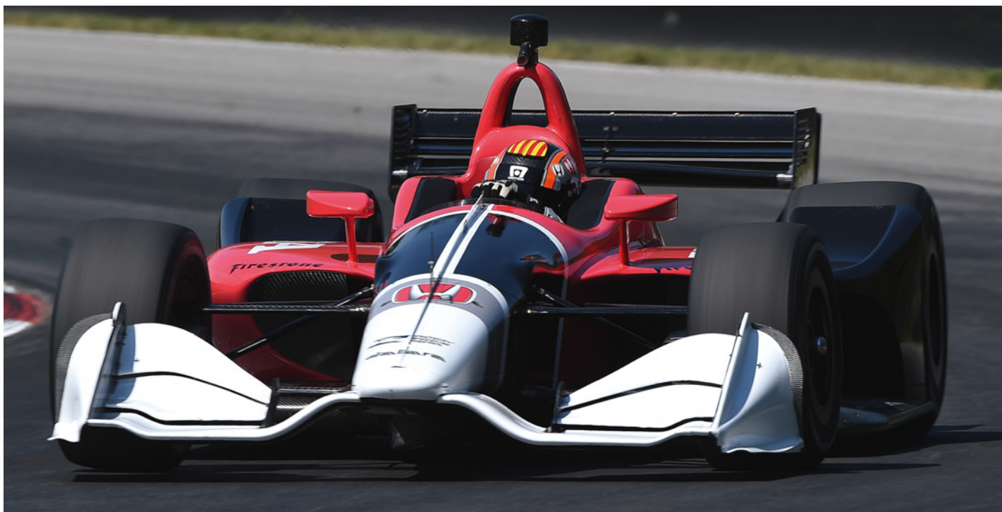
New road course aero package is capable of generating 5300lbs of downforce, which is a step down from the amount generated by the manufacturer kits; around the 6800lb region
