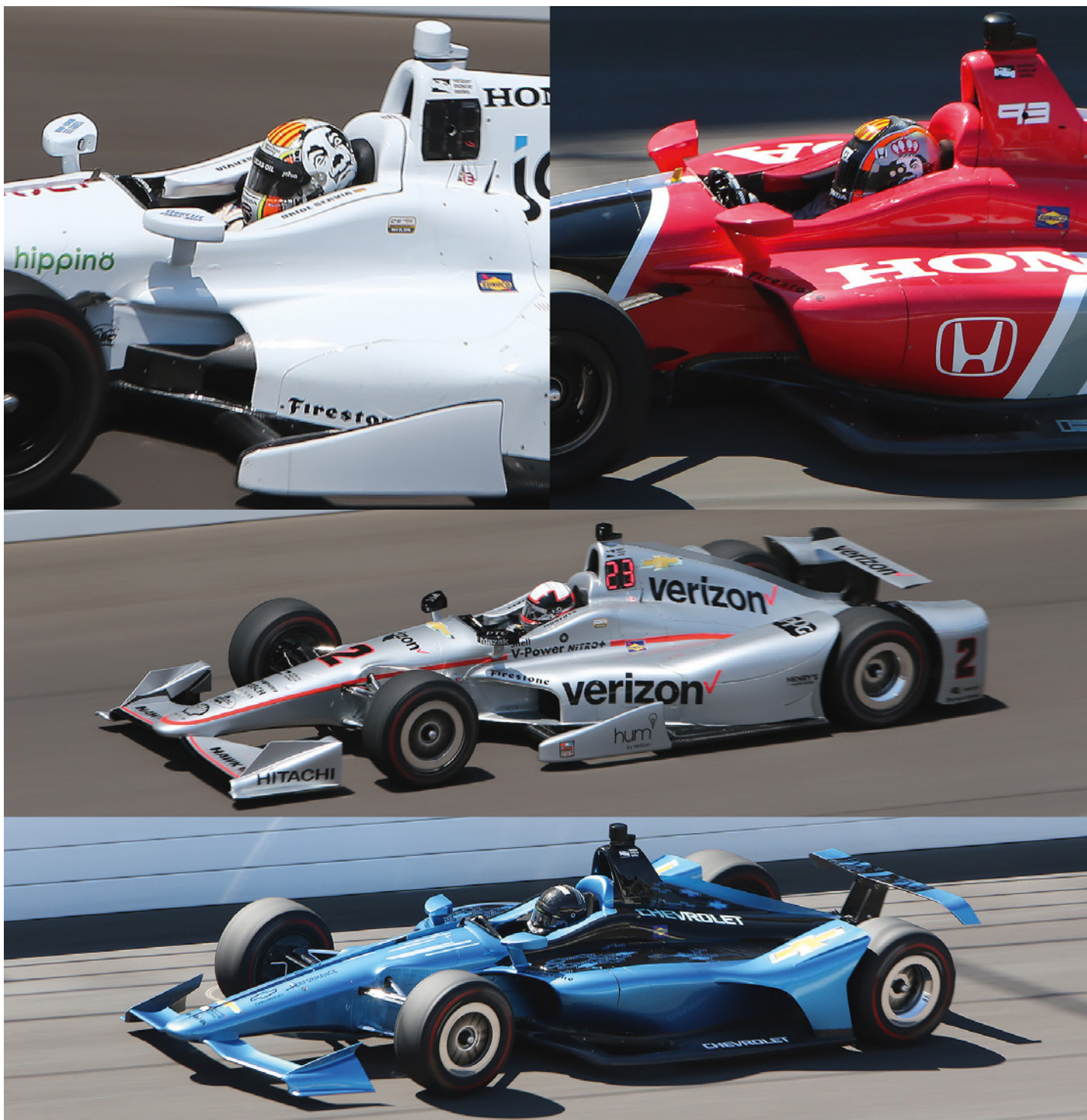
Top pictures: The difference between the sidepod leading edge treatment on this year's version of the DW12 (left) and the new bodykit. Bottom two pictures show the super speedway configuration of the new and old (top) kits. IndyCar was pleased with the way the racecar performed at the Indianapolis 500 this year and wanted to retain a similar aero performance
