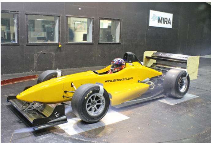
The DJ Firestorm was subjected to front wing tests in the MIRA full-scale wind tunnel
