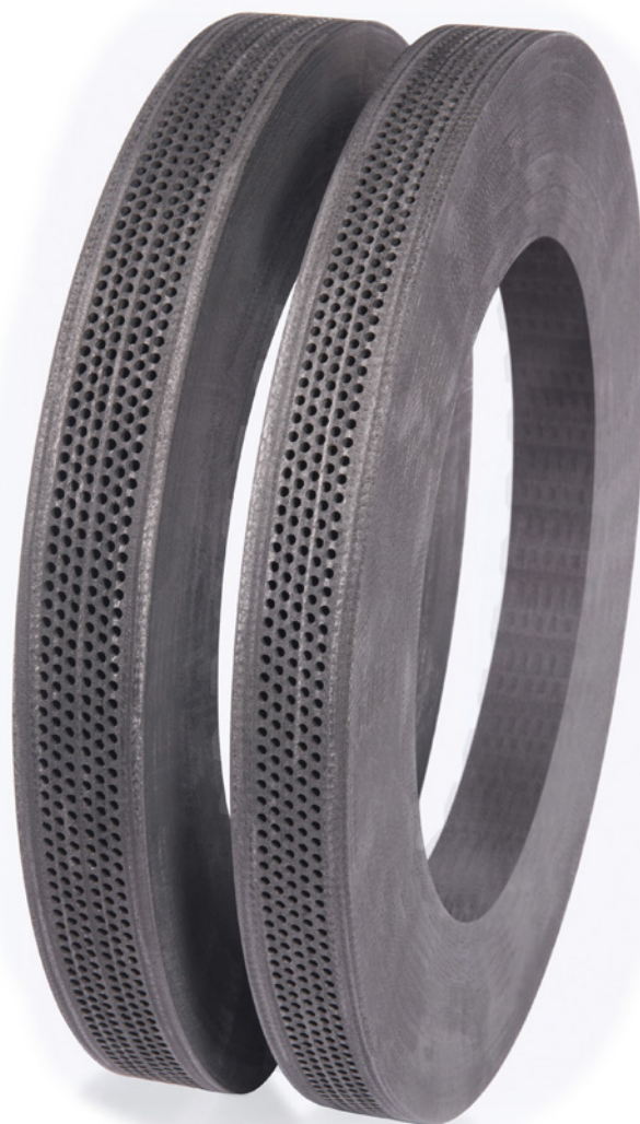
F1 carbon brake discs can reach 1200degC. That's why each disc can have up to 1300 ventilation holes in it to help to dissipate heat
