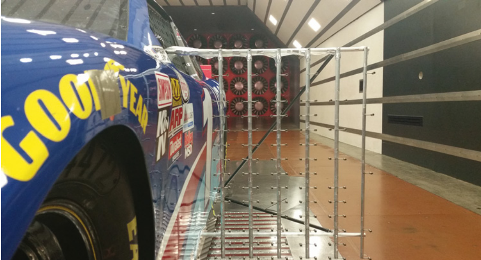
The accuracy of the CFD-predicted wake change was assessed by fitting a Kiel probe array to the racecar in the wind tunnel
