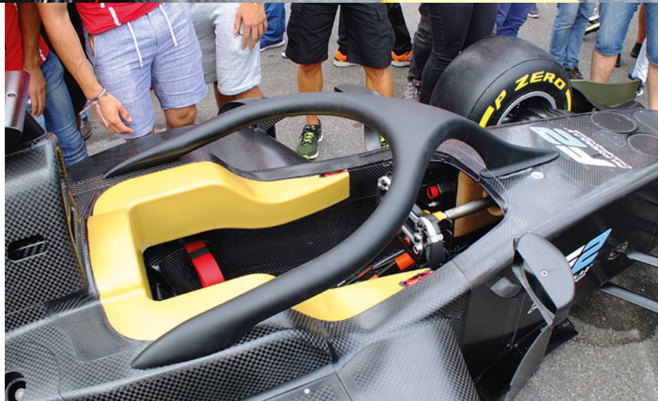
Above: The cockpit features extra Zylon panels which has had the knock on effect of increasing the car's weight. It has also been designed so that taller race drivers can be accommodated Right: The Halo fitted on the launch car was actually a dummy. The car was not originally going to include the new safety device and Dallara has had to design-in extra hard points on the chassis
