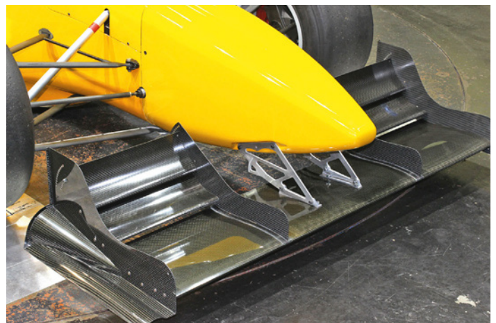
This two-flap arrangement was compared to the baseline single flap set-up on the car
