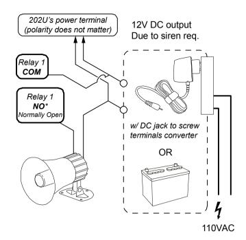
Shared power sources is not recommended for motor or other electronics which introduce noise into power line. Although 202U doesn't care about polarity, your target device may care, so inspect wiring carefully before power up.
