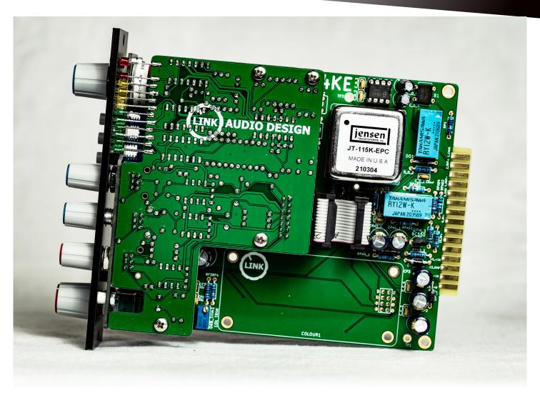
After finishing try to run an Audio Signal thru the Unit and try all switch modes, if everything works fine. In the next step we will calibrate this wonderful Preamp.
