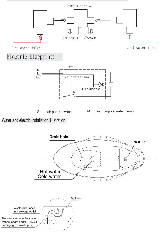
During installation, please avoid cutting the waste pipe with  $s \ensuremath{\mathsf{sharp}}$  objects (e.g. knife).
