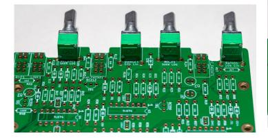
After having one pin of each pot soldered we add the bracket. The direction of the bracket is shown in the picture below. After having all pots screwed to the bracket, we can solder all pins, then we need to cut the pins. I cut all the pins before soldering, then they look better, but you can also cut them afterwards. Then unscrew the board from the bracket again.
