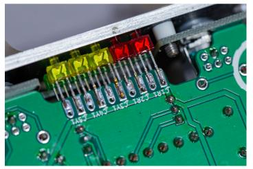
Once all solder points are done, remove and unscrew the Frontpanel and bracket again, we need that for next step.
