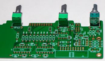
Check the alignment of the switches and pots from the upside again and try to bring them in line like the silkscreen is printed. After that install the blank bracket on the upper subboard and solder the pots in place.
