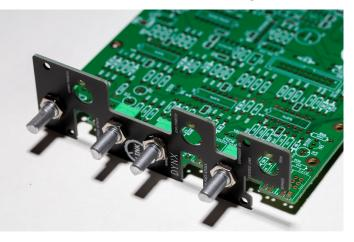
The next step is focusing on the pots and switches of the upper subboard, we can solder all pots and switches. Make sure to press them flush and firm to the poard and fix them with one solder point.
