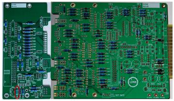
After Placing and Soldering all Resistors, we solder the next bigger parts like IC-Sockets, VCA-Socket Bridge Rectifier and small Capacitors, like 100nF and 22pF.
