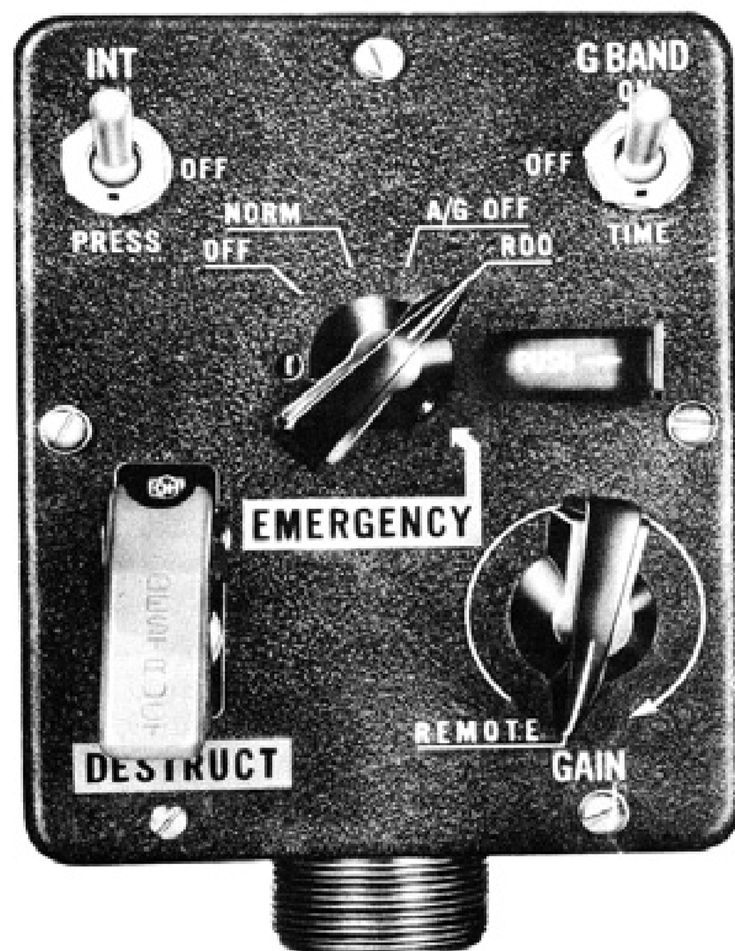
Figure 72 — IFF Pilot's Control
