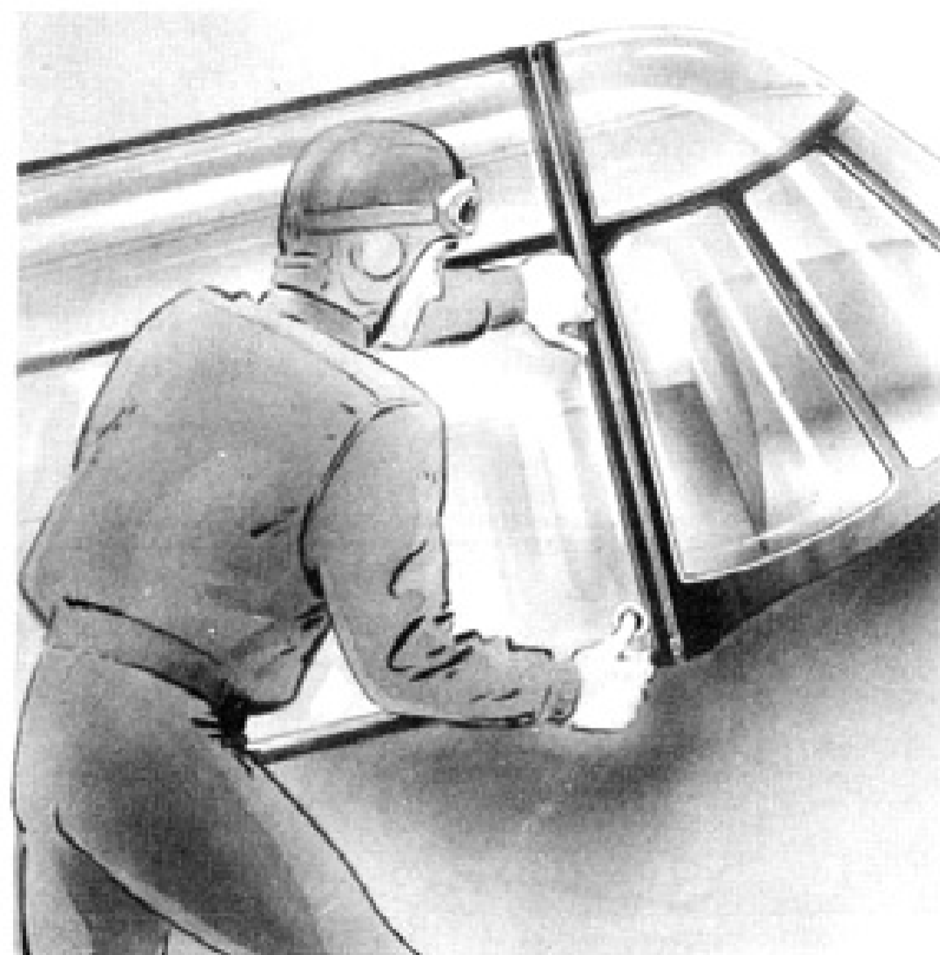
Figure 43 — Access to Cockpit
