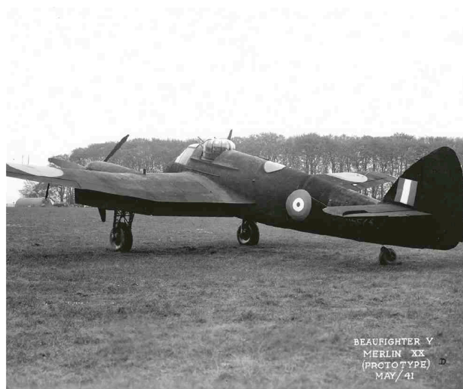
The first of two Mk IIs, converted to Mk V standard with a Boulton Paul turret mounted behind the pilot's cockpit. Installed in an effort to improve the aircraft's field of fire, the cumbersome turret reduced the performance of the Beaufighter and the idea was abandoned.
