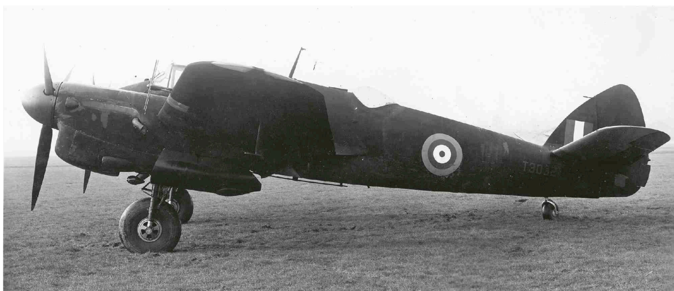
After initial service with the FIU, Mk IIF T3032 proved to be a useful trials machine on which the familiar dihedral tailplane was tested and later the large dorsal fillet which was adopted by the Mk X.
