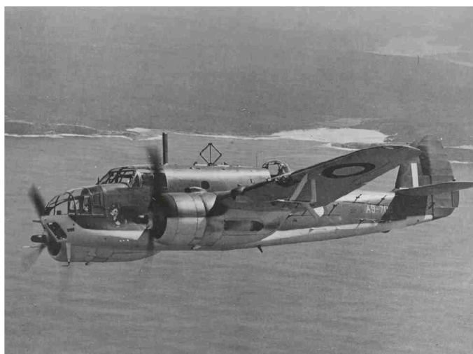
▼ The first production Australian-built Beaufort Mk VIII which was powered by a pair of license-built Pratt & Whitney S3C4-G engines with Curtiss Electric propellers. The aircraft also featured larger fuel tanks and Loran navigation system. 540 were built and production did not come to an end until August 1944.
