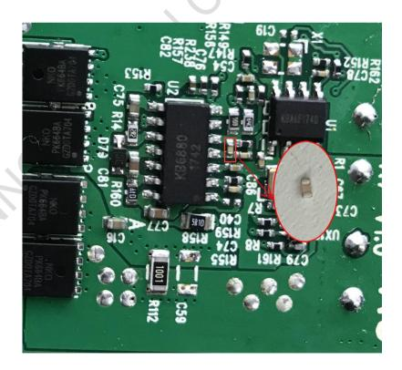
5. When the two ends of the components melt, clip out the components with tweezers, and remove the air gun. Pay attention to check whether unbiased,
