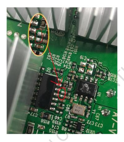
6.After taking the components off, you can put the board back into the barrel, make sure that components in three hashboards have all been fixed. Put the fan back, lock the four fixed screws, eventually the components are fixed.
