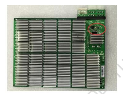
4.Heat the gray rectangular capacitor in the picture below with air gun (Adjust the air volume of the gun to the minimum, to the temperature of about 380 degree centigrade, keep the air gun 1cm from the element, heat for about 30 seconds) .If the corresponding location do not have the component, then no fix is needed, put it back to the machine.
