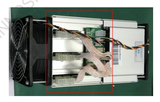
2. Removal of fan bracket: remove the 4 screws from the fixed fan bracket (at the four corners of the fan bracket, 2.8mm tip self-tapping screw)
