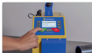
Start welding. Perform the required controls (alignment, depth of insertion and fusion indicators).
