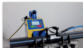
Start welding. Perform the required controls (alignment, depth of insertion and fusion indicators).
