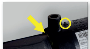
Start welding. Perform the required controls (alignment, depth of insertion and fusion indicators).
