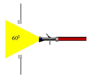
Fig 4: Ventilation using a branch
