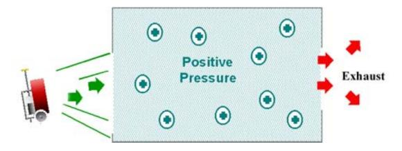
Fig 5: Principles of positive pressure
