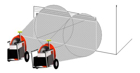
Fig 8: Using two fans on a large opening
