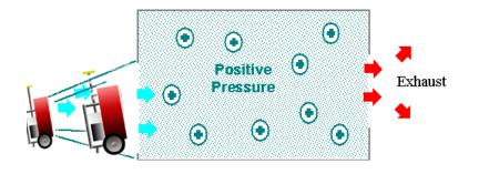
Fig 7: Using two fans inline
