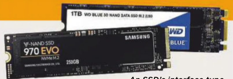
An SSD's interface type is usually written on the module – just check what your PC can accept
