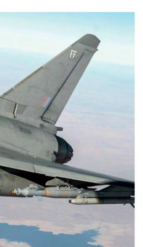
Armed with four Paveway IV laser/GPS-guided bombs, and fuselage-mounted AIM-120 and underwing ASRAAM air-to-air missiles, this Typhoon was taking fuel from a USAF KC-135 tanker over Iraq on December 22, 2015. US Air Force/Staff Sgt Corey Hook
