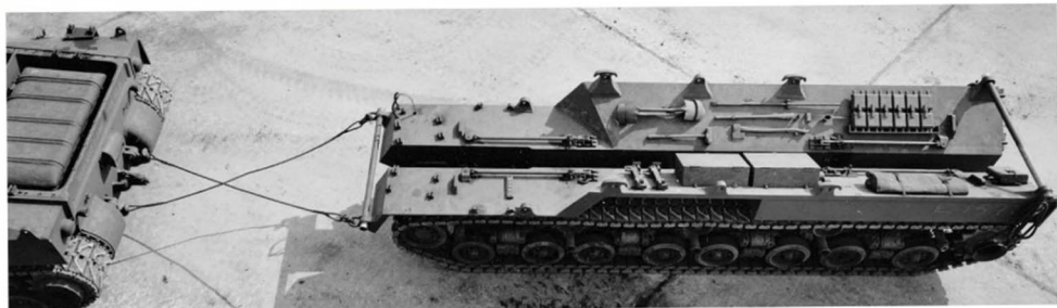
An overhead view demonstrates the manner in which the outer track units were attached skirt-to-skirt to form an assembly that the T95 could tow. The unit was relatively narrow and was intended for towing on flat, solid surfaces. Note the steel tubes that helped to hold the units together, at the front and rear of the assembly.
