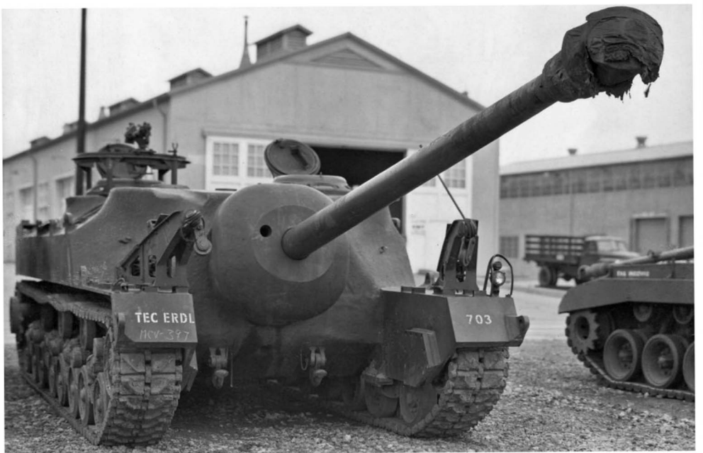
Above: A front view of a T28 with its outer tracks removed at Aberdeen Proving Ground in March 1951 displays how the 105mm gun exited the fighting compartment. Two tow hooks are visible towards the bottom of the hull front. On the face of the mantlet on the right side of the gun is the aperture for the gunner's direct sight; he also had a periscope on the hull roof.
