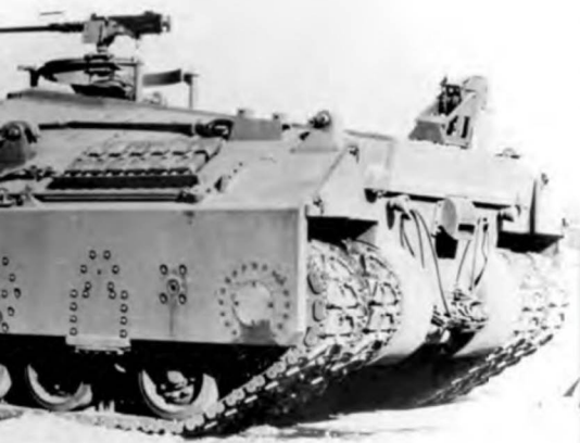
Below: The second T95 pilot is rigged to tow its conjoined outer track units at Aberdeen Proving Ground in March 1946. The right unit is visible in this view, and the skirts of the two units were joined face-to-face in the middle. Details of the HVSS bogie assemblies are visible. The two men to the right are demonstrating the braking arrangement of the rope wrapped around the drum on the sprocket.
