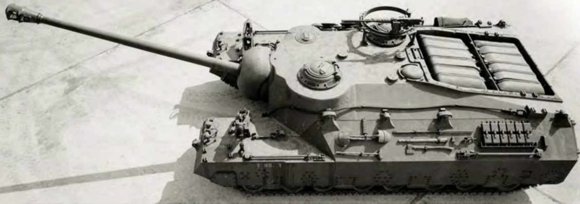
Above: As seen from overhead, the gun mount of the T95 was at the very front of the hull. Here, both of the small cranes for lifting the outer track units to the side are attached to their brackets above the left and right front fenders. The brackets for mounting the cranes toward the rear of the T95 are visible on each side of the transmission compartment cover. The pioneer tools are also in view. Right: Photographed in January 1946, the number one prototype has 'T 95. 1' stencilled in white on the skirt. Poised over the front fender and on the rear of the vehicle are two small cranes for removing and reattaching the outer sections of tracks and suspension. A .50cal machine gun ring mount is fixed above the commander's cupola.
