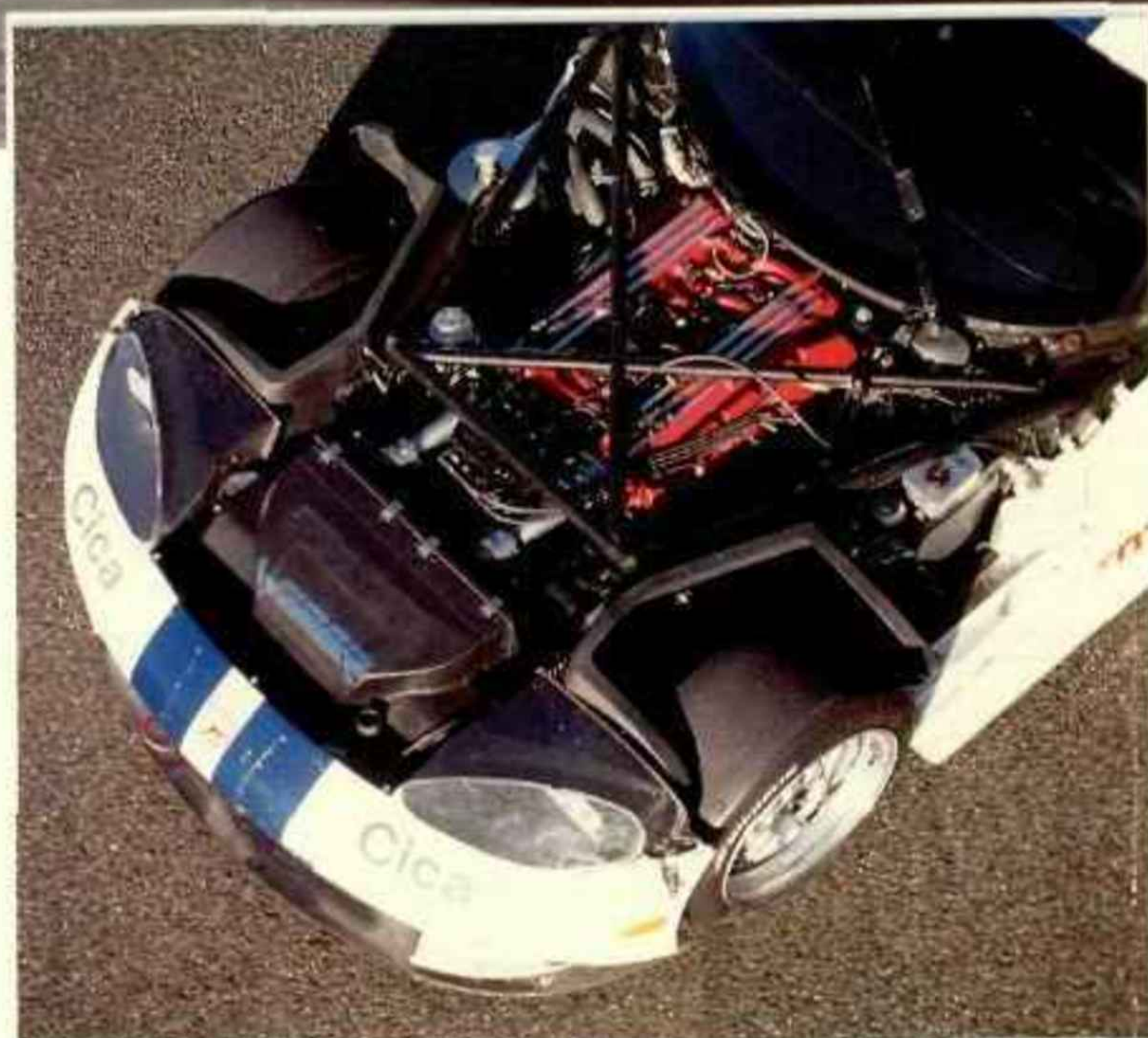
GTS-R puts out 700bhp from its 8-litre V10 and, with a minimal downforce setting, will reach 220mph
