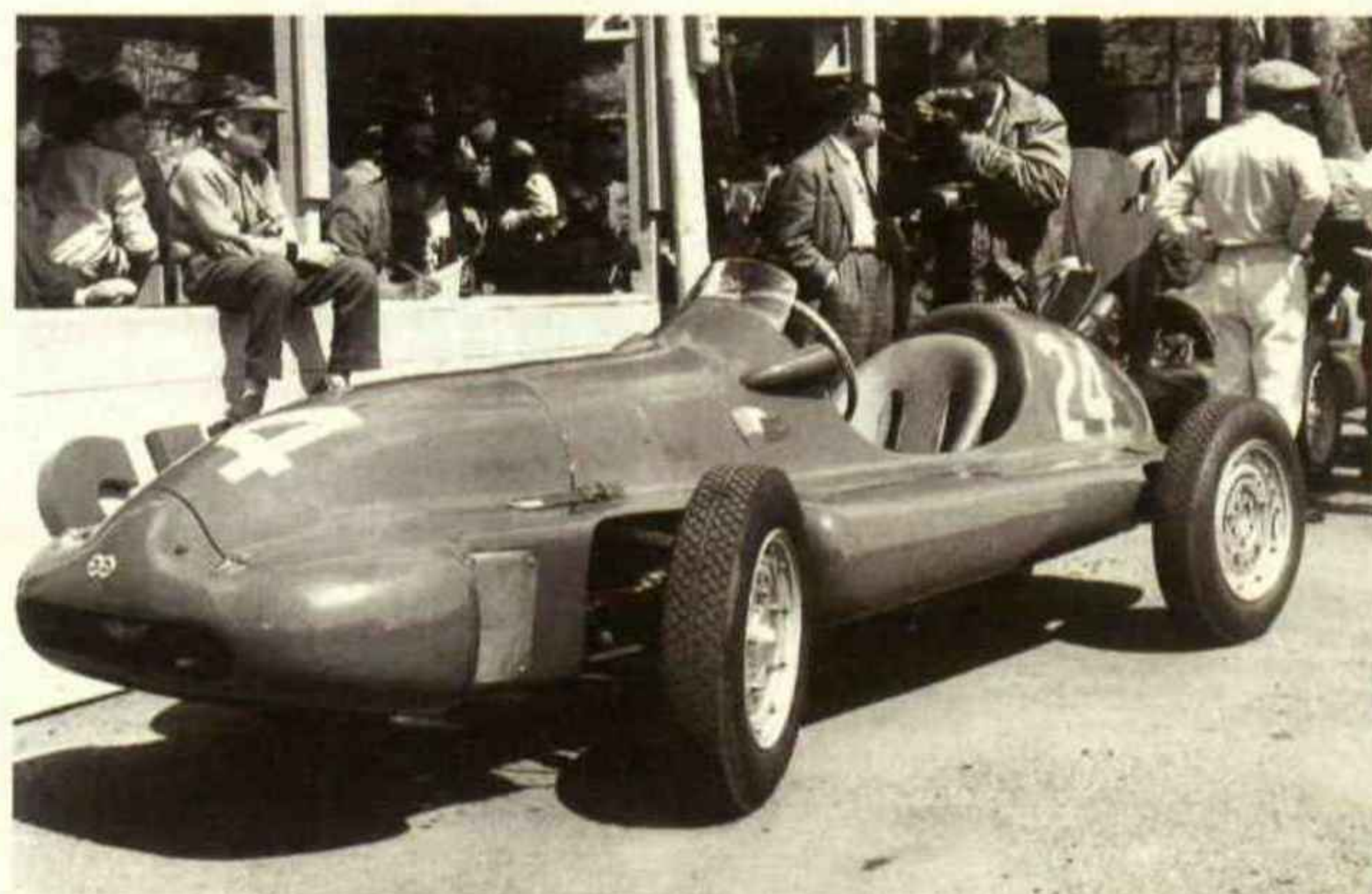
Technically interesting, the Cisitalia-Porsche (above) used a mid-mounted supercharged flat-12 and four-wheel drive which could be switched into rear drive. Nuvolari tried it (left) but the project was too ambitious and Cisitalia ran out of money. Outlandish DB (below) was front drive but was also fatally under-powered and terminally over-weight
