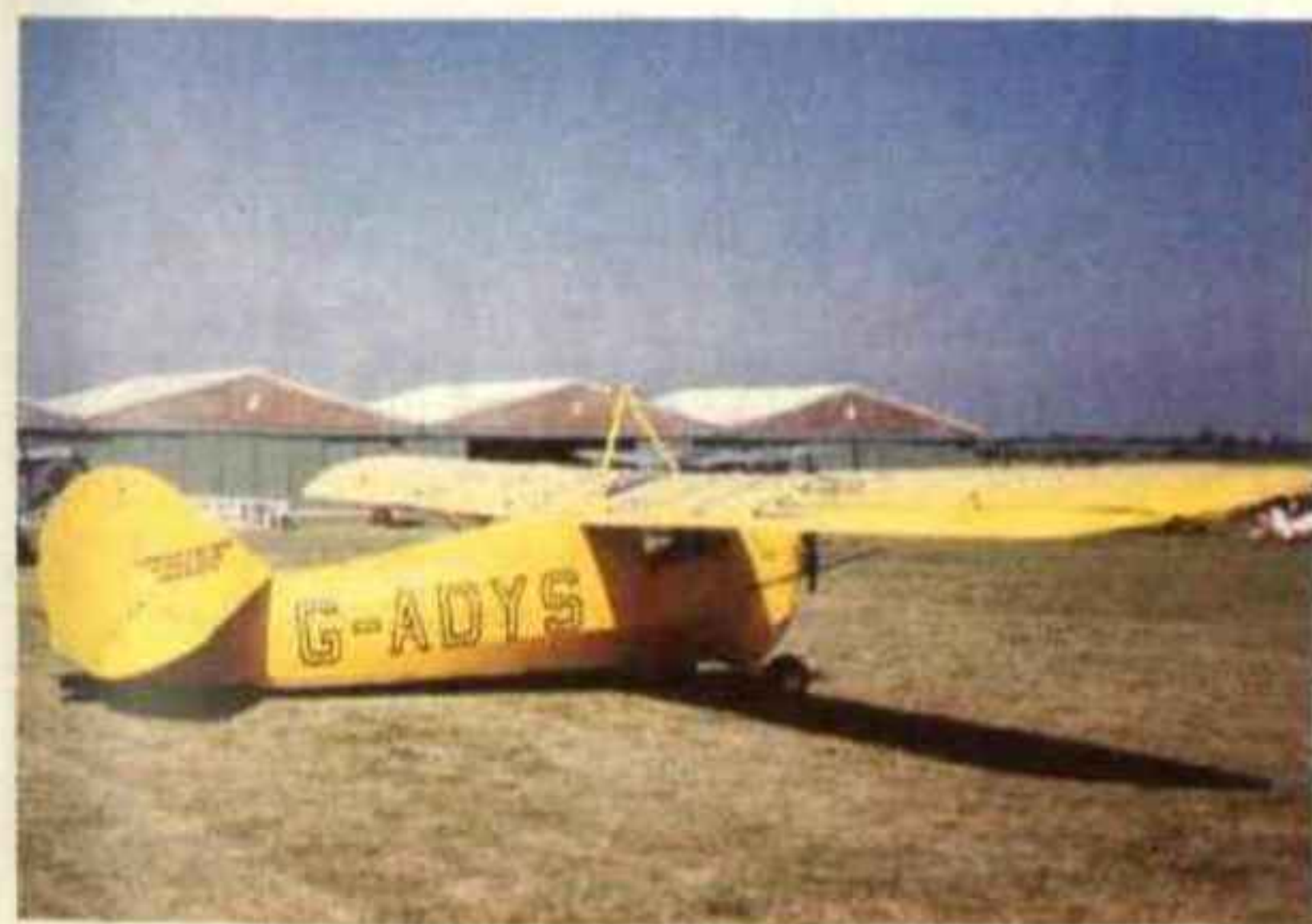
The Cooper's Aeronca C3 is one of three still flying in Britain: 70mph, two up on 2 1/2 gallons per hour
