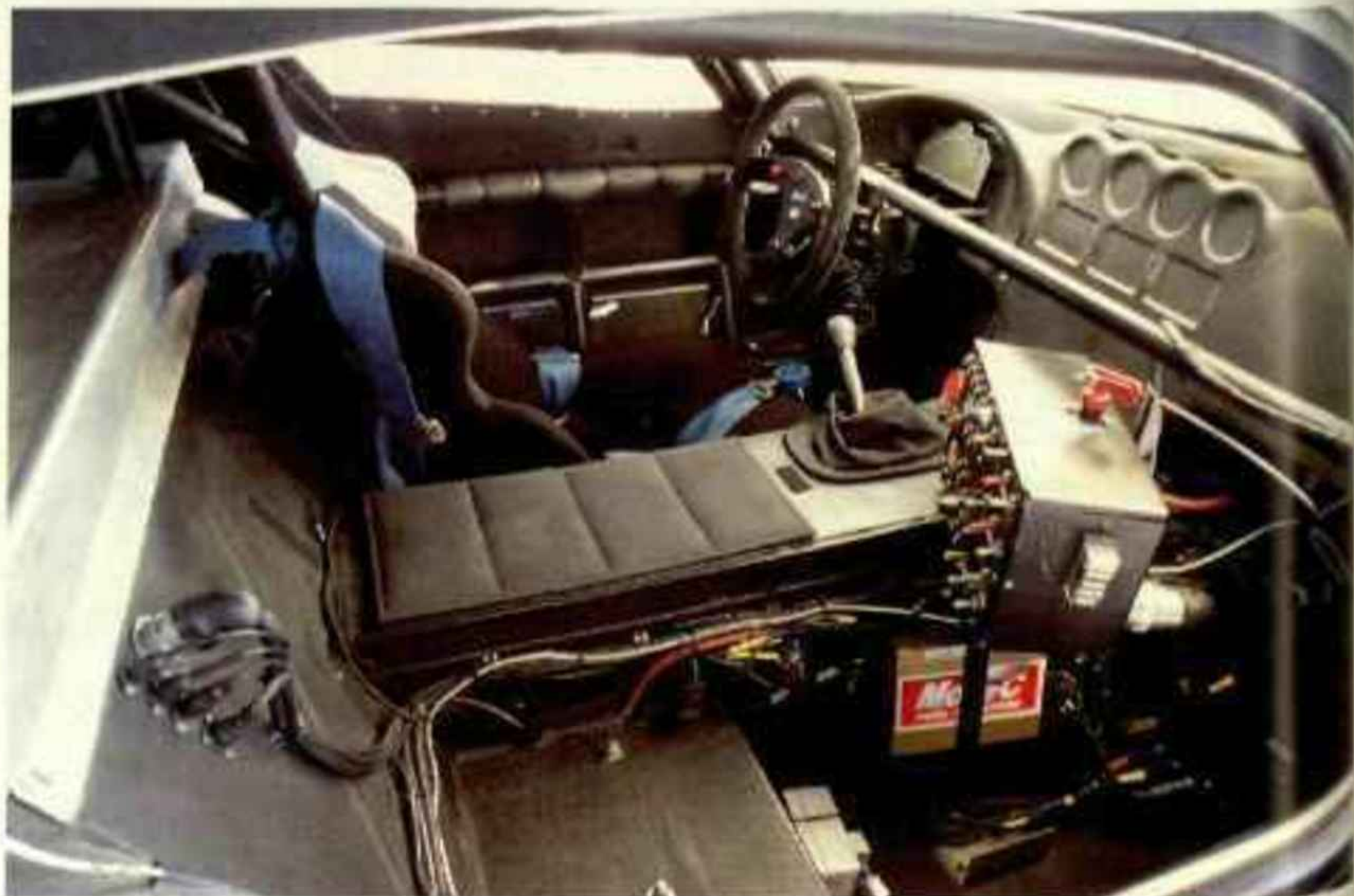
All functions are actuated by the black box located beside the road-based, slower shifting six-speed gearbox
