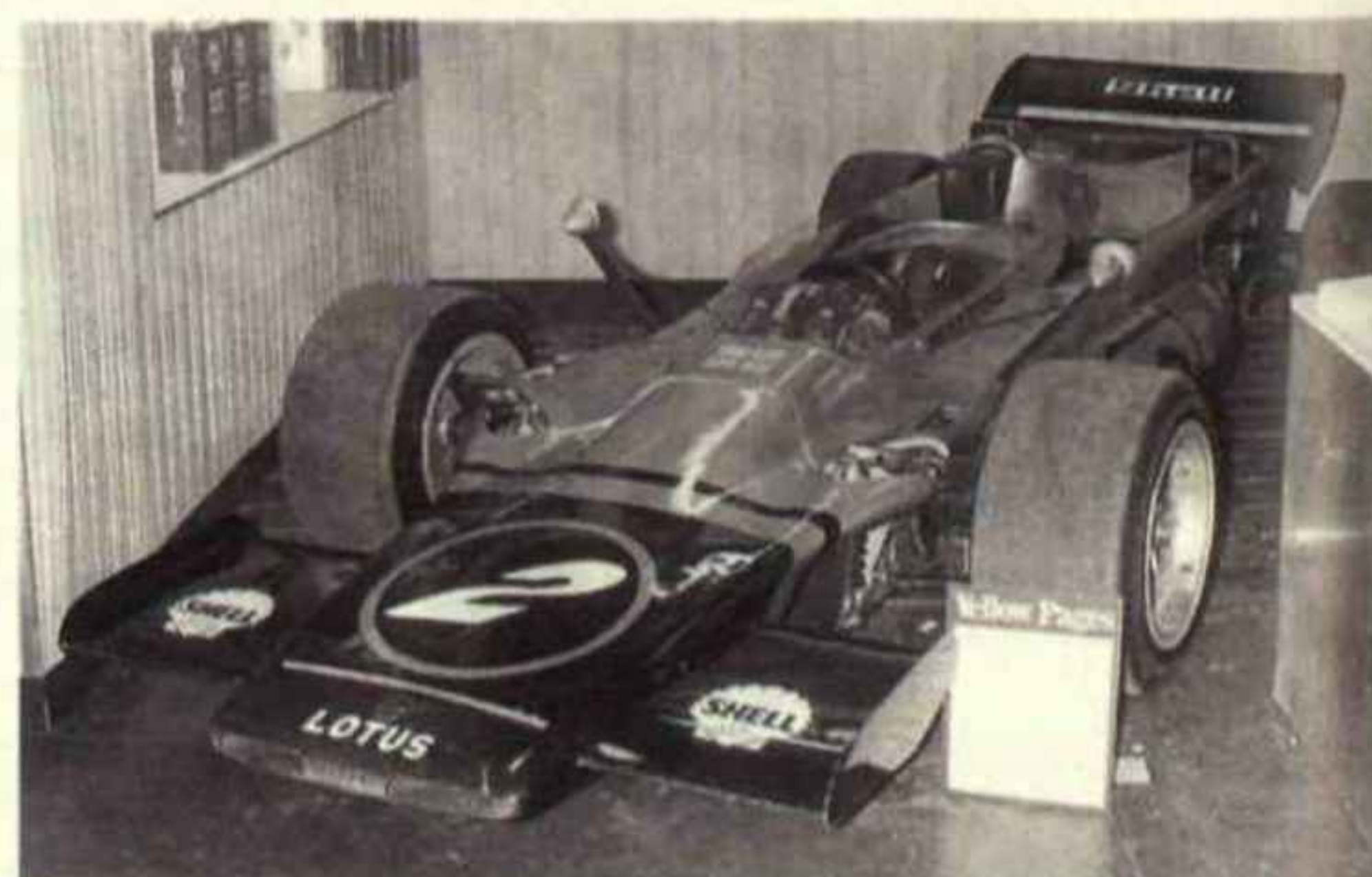
The American Scarab team (above) was a victim of bad timing, just as BRM was the victim of a bad idea with its H16-engined effort (in foreground, left). The gas turbine-powered Lotus 56B (below) had woeful turbo lag. Four-wheel drive didn't save it
