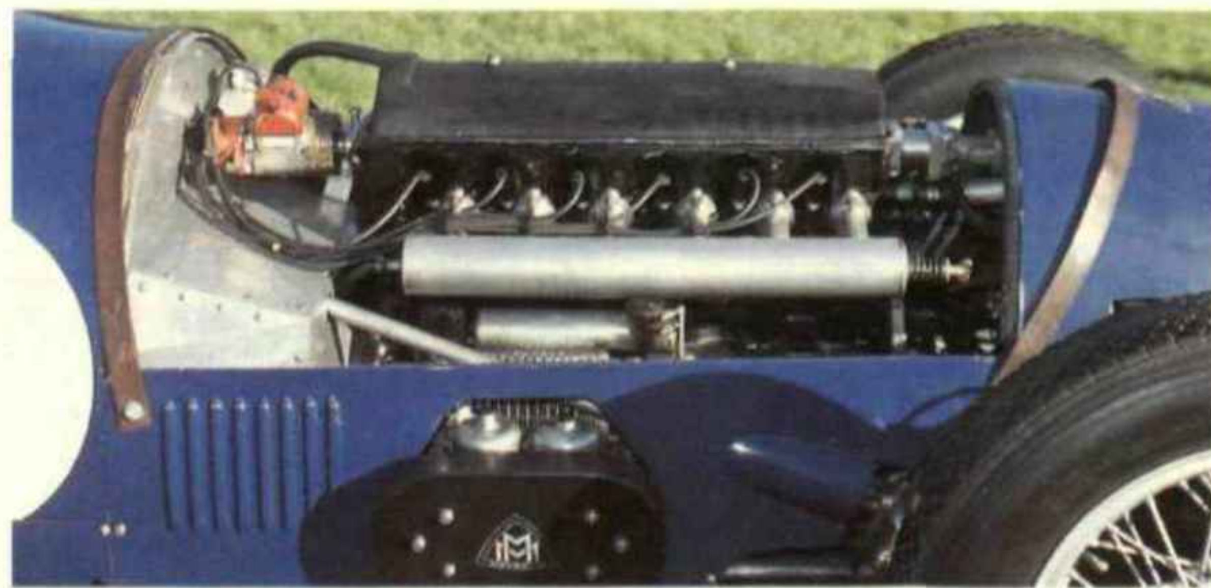
In supercharged form blower sits low beside engine, with two big carbs
