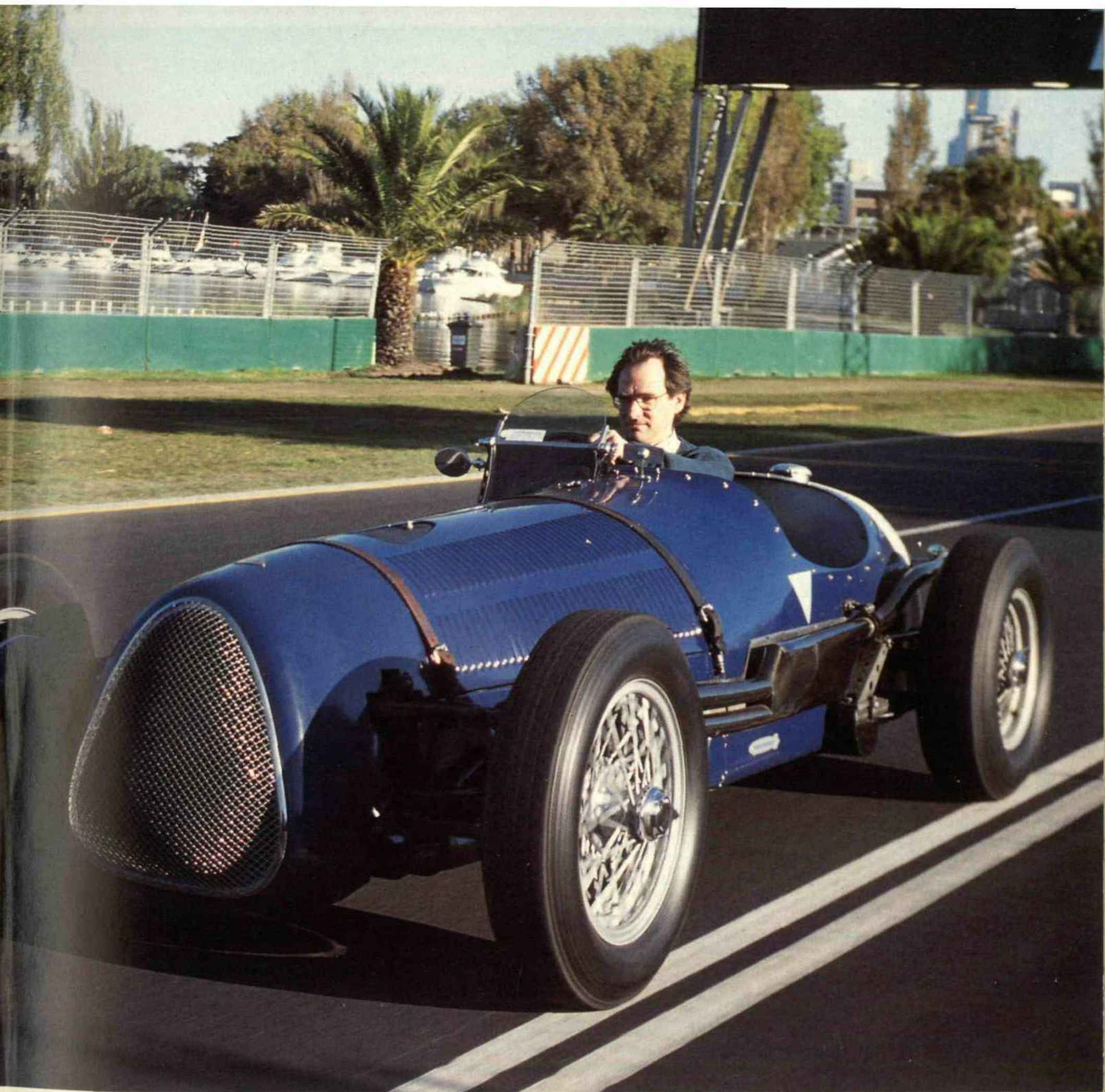
In Maybach I form, car was a nominal two-seater, with driver squeezed in beside transmission. Original Fiat gearbox long since replaced by Jaguar Moss 'box to cope with big six's huge torque
