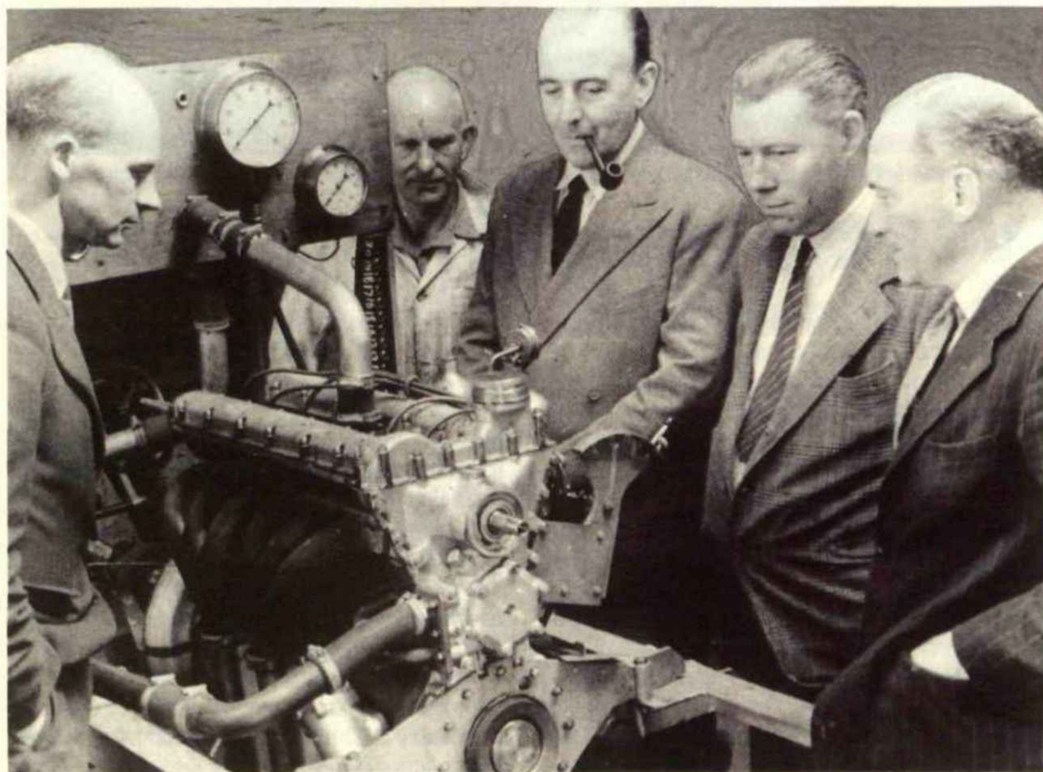
W O watches the birth of another one of his legends: the LB6 engine that powered Feltham Astons until 1959
