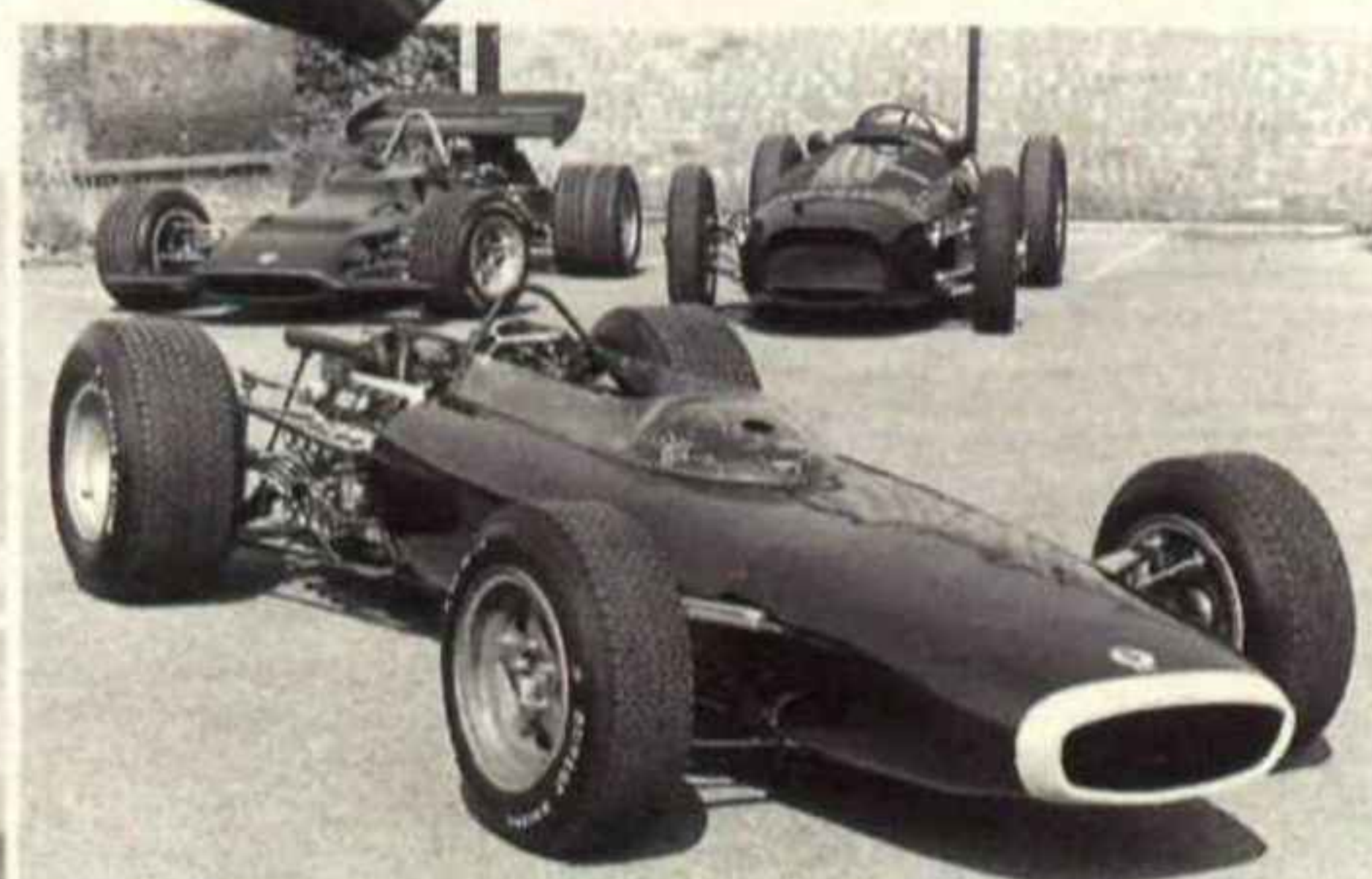
The American Scarab team (above) was a victim of bad timing, just as BRM was the victim of a bad idea with its H16-engined effort (in foreground, left). The gas turbine-powered Lotus 56B (below) had woeful turbo lag. Four-wheel drive didn't save it
