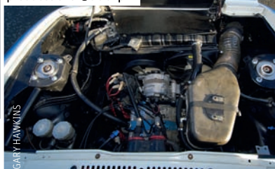
1308cc rotary engine produces over 300bhp
