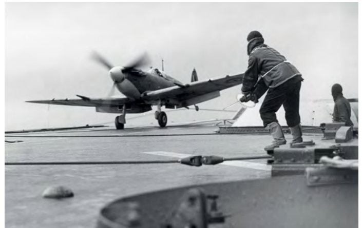
A deck batsman guides in a Seafire for a successful arrested landing. The photo's caption states the aircraft carrier was HMS 'Indomitable'. Due to the poor forward view, landings aboard carriers would normally be made using a banking approach, to keep the flight deck in view for as long as possible.
