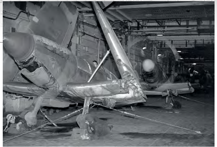
A Seafire Mk.III with wings folded has its engine run up while apparently undergoing maintenance on the hangar deck. Note the two groundcrew bracing the wheel chocks to prevent the aircraft from moving forward. The Mk.III introduced a four-bladed propeller unit (Roto/Jablo) as standard.
