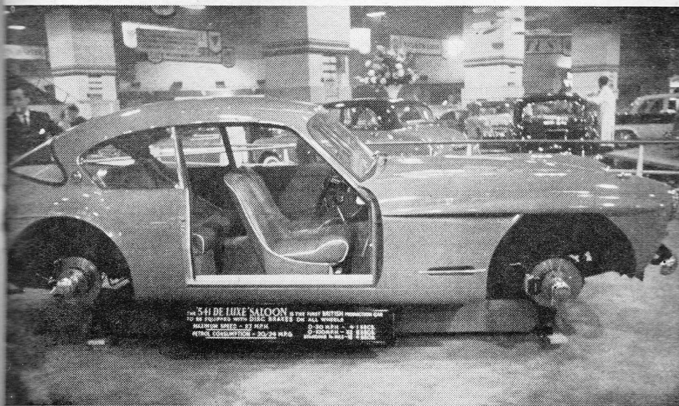
FIRST British production car with disc brakes on all four wheels is the shapely Jensen "541" de luxe (left). The body is of plastic.
