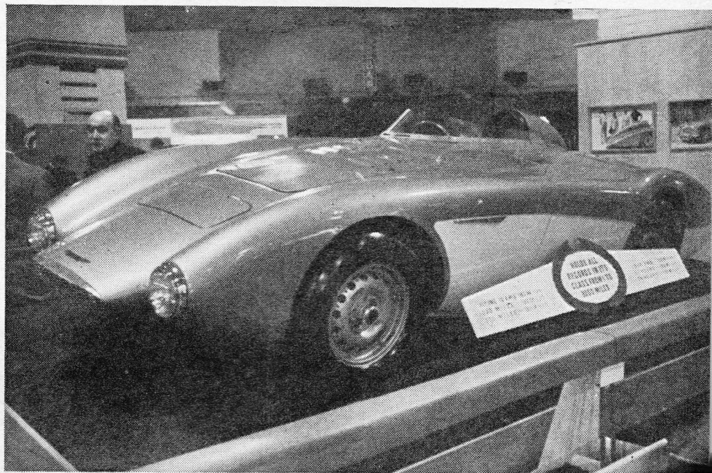
SOUND HEART for the new Allard Palm Beach Mk. II (above) is provided by the 3 1/2-litre Jaguar engine. The tubular chassis embodies independent front suspension by wishbones and laminated torsion bars. At the rear, the rigid axle is suspended on large helical springs. An optional power unit on this model is the 2.6-litre Ford Zephyr II.
