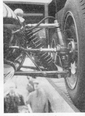
NEW Oleo-strut front suspension as used on the new Lola. It was not raced at Aintree.
