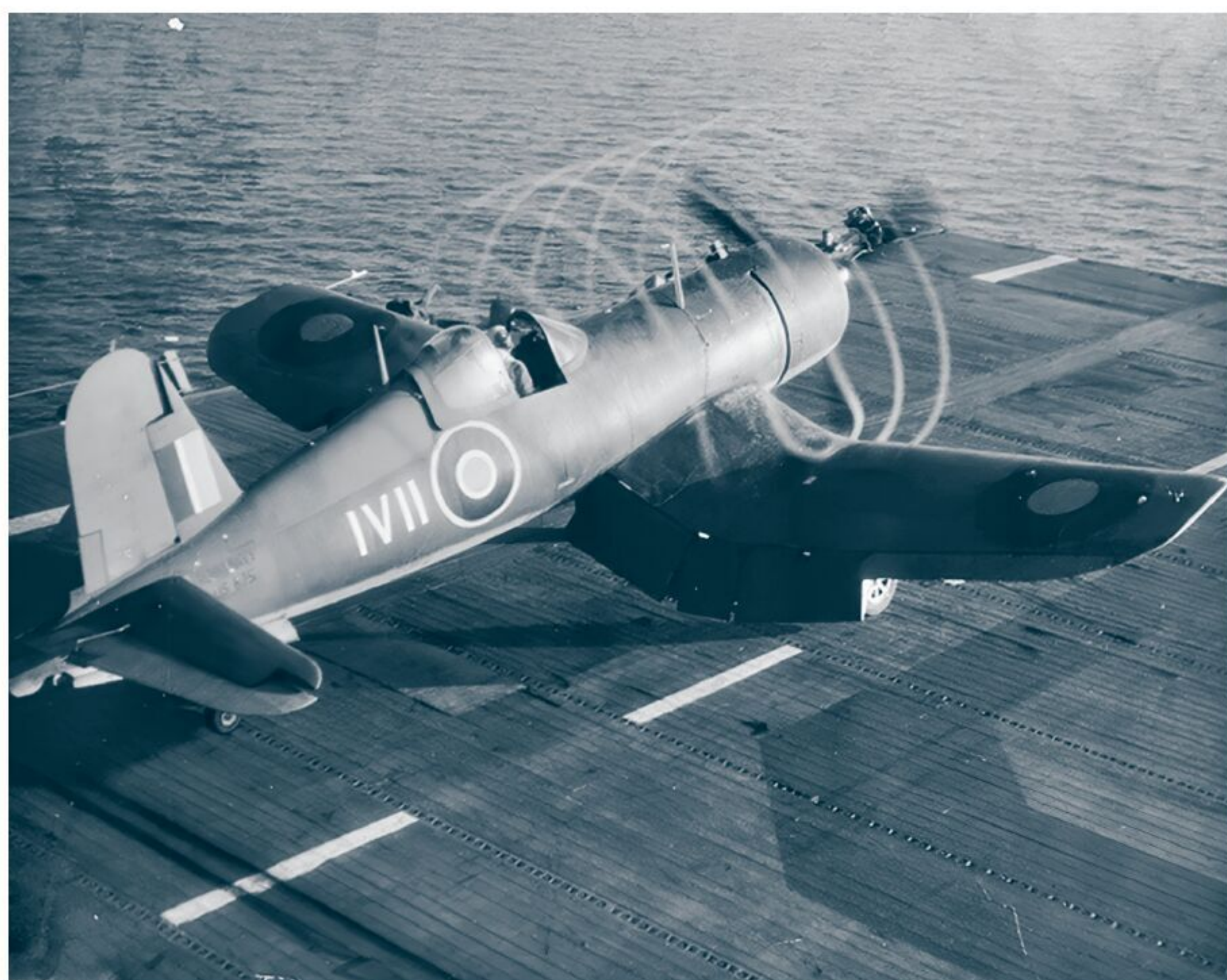
A Goodyear produced FG-1D Corsair IV, 1V11 of 1835 NAS, generates impressive vortices from the huge propeller on takeoff during a carrier training session. (Photo author's collection)
