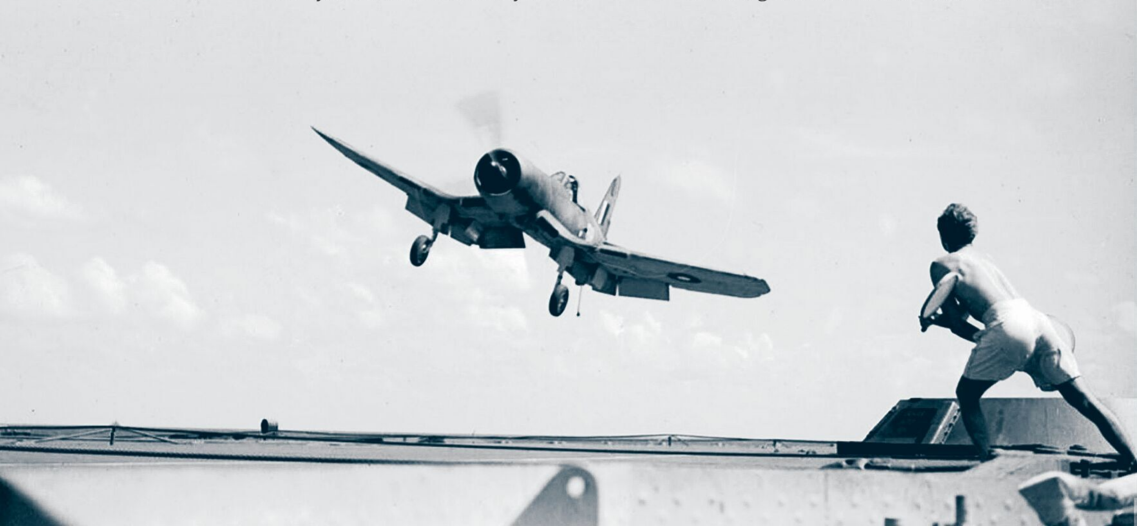
Demonstrating the curved approach needed for deck landings in the F4U, this FAA Corsair JT358, landing on HMS Illustrious in the Indian Ocean in May 1944, still has bank applied as the Deck Landing Control Officer signals the "cut" with his bats. (Photo author's collection)
