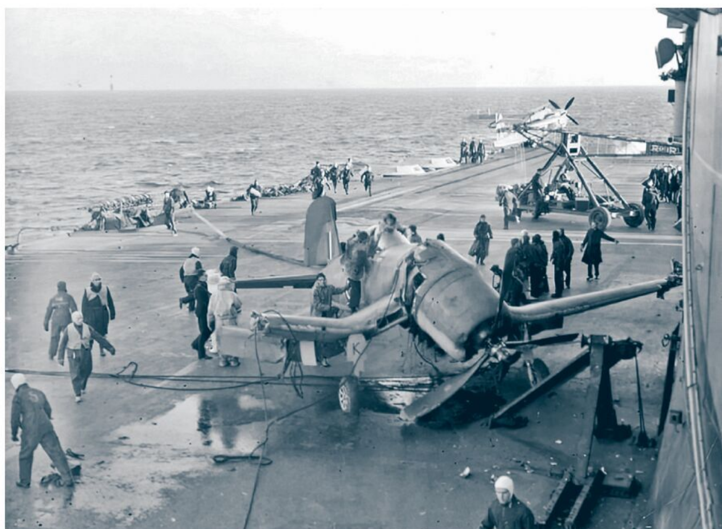
Corsair JT210 ("K") of 1830 NAS, flown by Lt. A. W. Sutton, RCNVR, missed the wires on landing on HMS Illustrious on December 9, 1943. After being arrested by the crash barrier, the aircraft careened into the carrier deck island, nearly tearing the engine from its mountings. (Photo author's collection)
