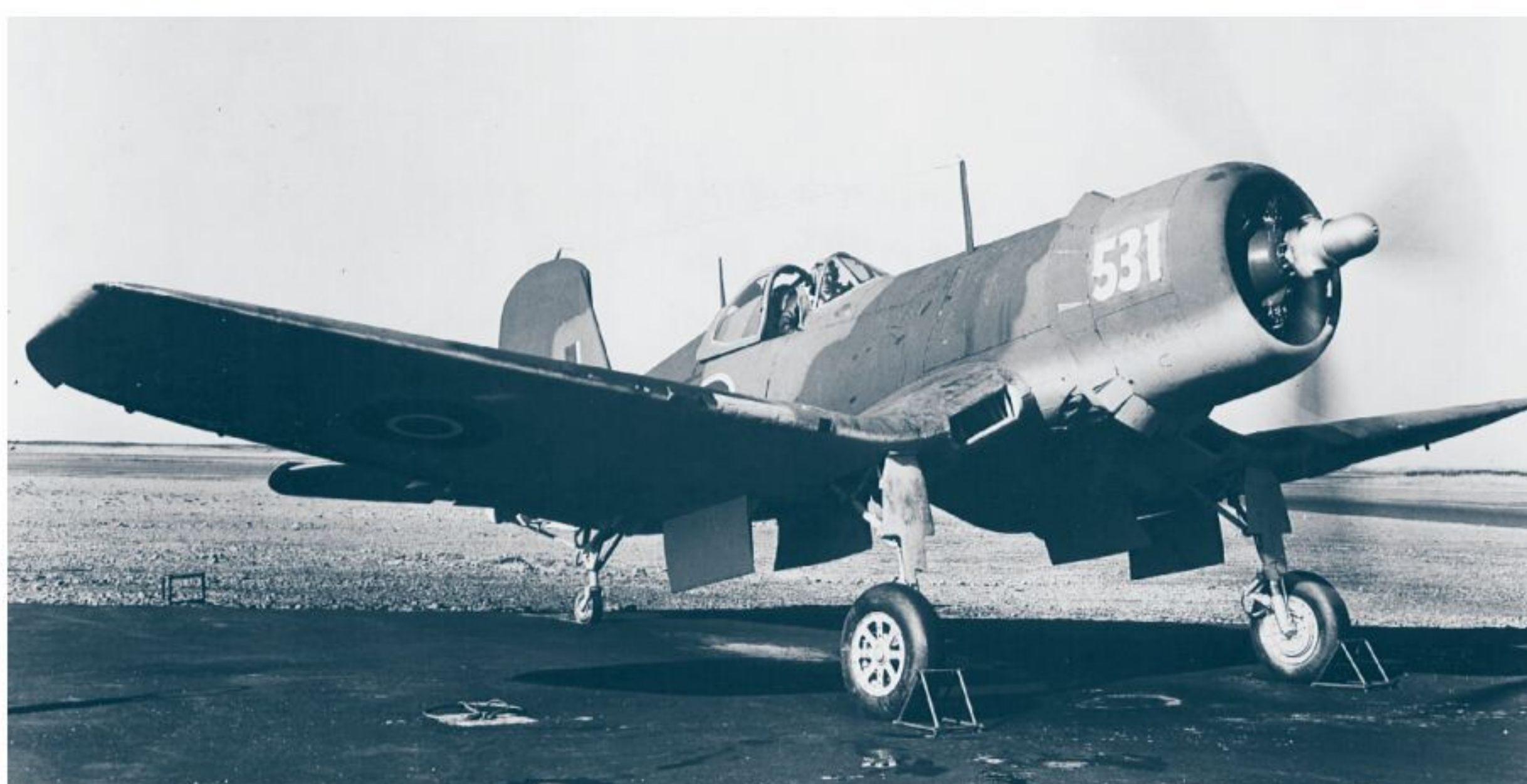
TOP: A Royal Navy Fleet Air Arm F4U Corsair 1 taxis at Roosevelt Field, Long Island, New York in 1943. The restricted forward view over the long nose from the aft-mounted cockpit is apparent in this view. (Photo author's collection)
