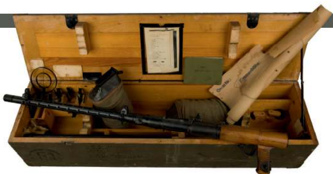
■ An MG15 in its transit case, complete with spares - including sights, tools and empty cartridge case collector bags.
