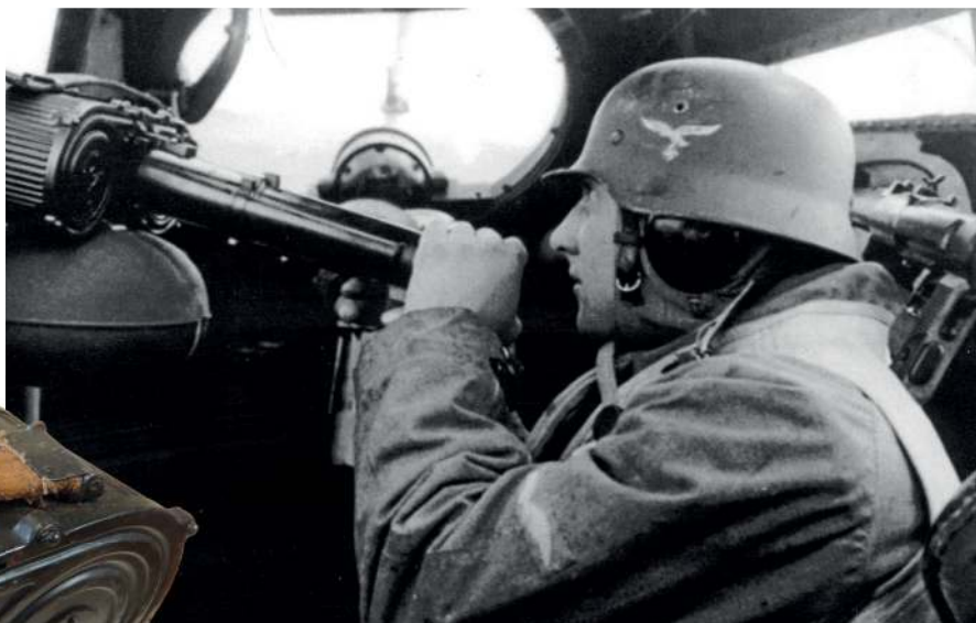
■ A steel-helmeted Luftwaffe crew member of a Dornier 17-Z mans one of the defensive MG15s fitted with a 'bowl' type empty case collector.
