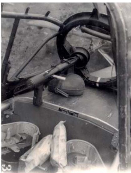
■ The MG15 in its rear position onboard a Junkers 87 Stuka. The gun is mounted in a ball-and-socket swivel in a rotatable gun ring, giving a wide field of fire. Spare saddle drums can be seen stowed in racks, and an empty case container is fitted underneath the gun.
