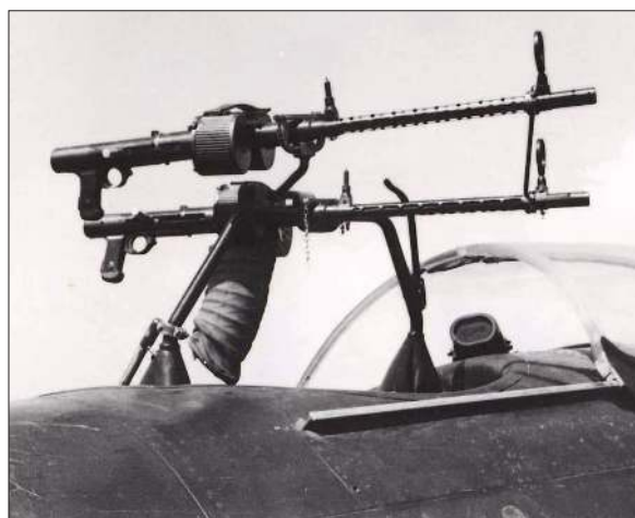
■ The double MG15 mounting fitted by Fritz Pons to his Heinkel 111 during 1940. Only one cartridge case collector bag is fitted. The empty cases from the outboard gun were allowed to fall overboard. (Left) Oberfeldwebel Fritz Pons of 8./KG55, 1940.
