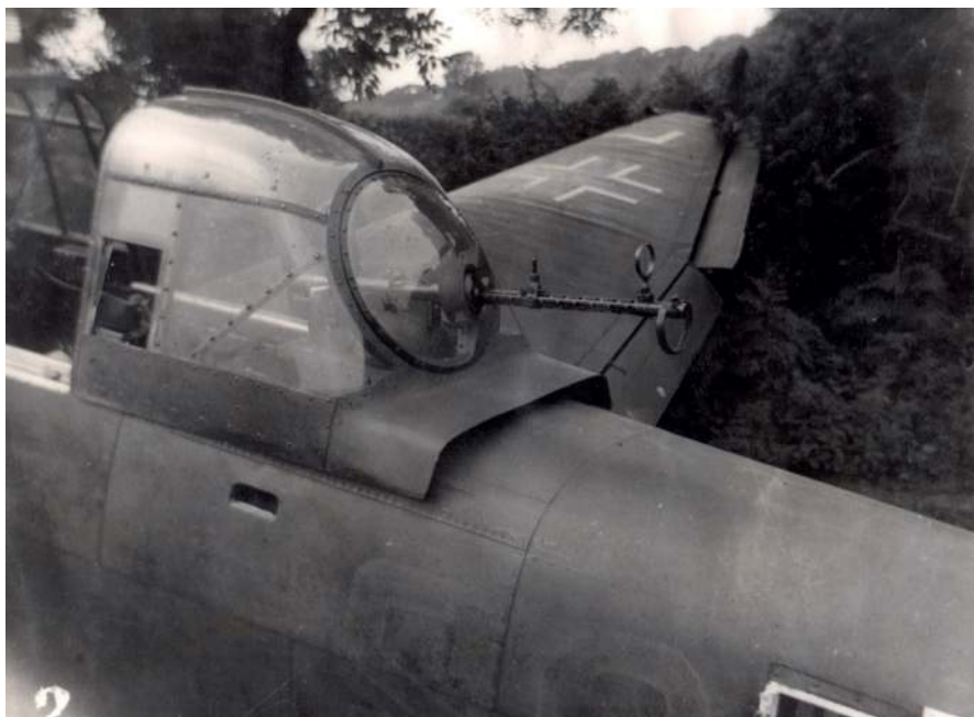
■ An external view of the same weapon, showing a device at the end of the barrel to prevent shots being fired into the gunner's own aircraft.
