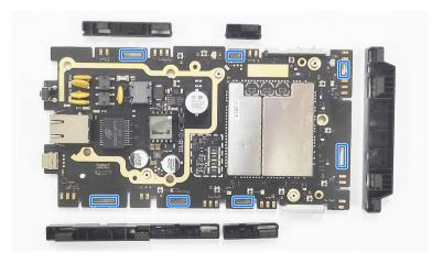
13. Remove the last 4 screws from the mainboard.
