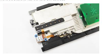
6. Remove the FPC (together with the LED and the nano-SIM card slot) from the front cooling support.
