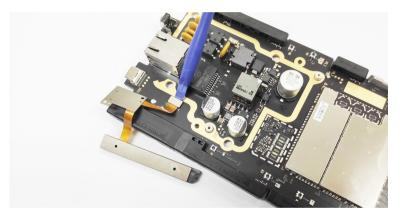
12. Unlock (positions of the locks shown below) the antennas and remove them from the mainboard.
