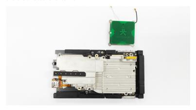
10. Remove the 4 screws from the front cooling support to separate it from the mainboard.
