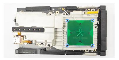
8. Disconnect the RF cables from the mainboard.
