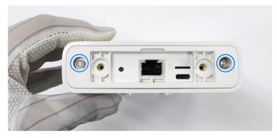
3. Draw out the inner assembly from the shell.
