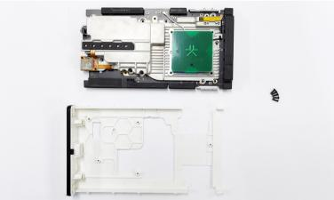
5. Remove the 2 screws near the nano-SIM card slot.
