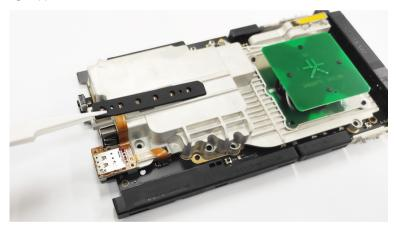
7. Remove the 4 screws on the corners of the directional antenna.
