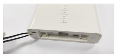
2. Remove the 2 screws under the patches.
