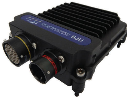
ABOVE EtherCAT is used to connect Cosworth's CLU and SJU
