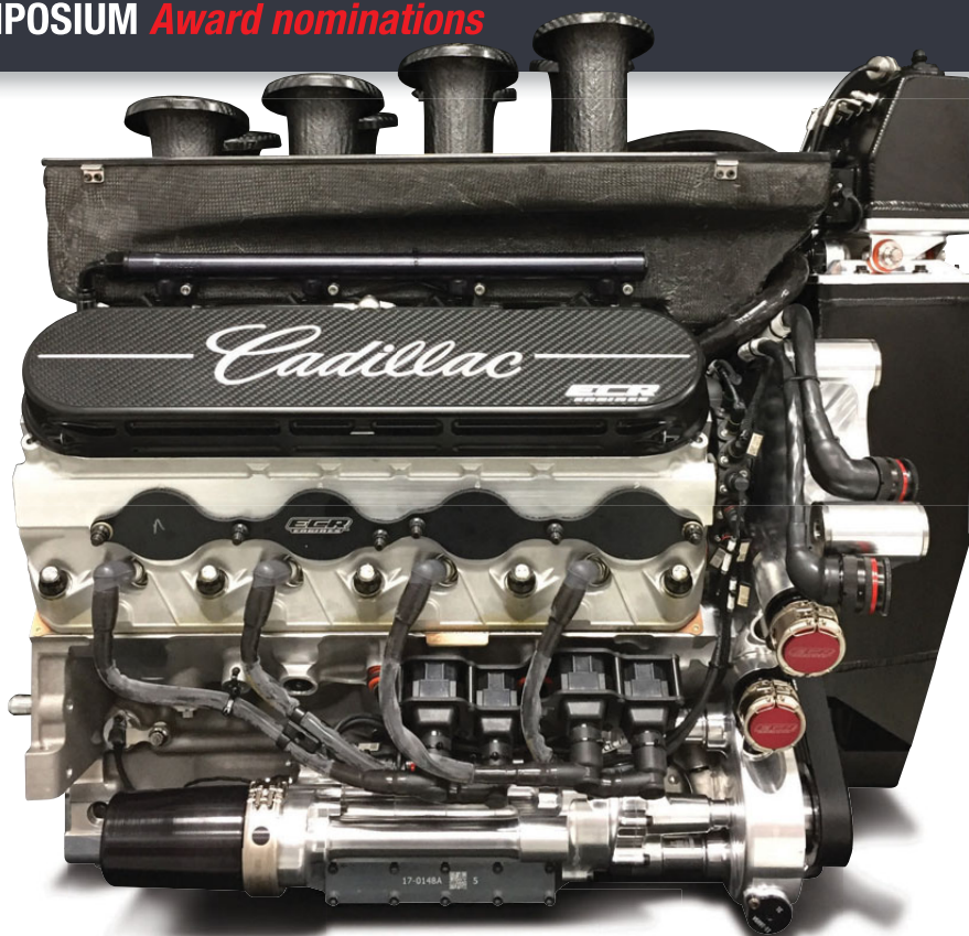
ABOVE The extensive NASCAR experience of ECR Engines, particularly in valvetrain development, underpins Cadillac's all-conquering 6.2-litre naturally aspirated V8
