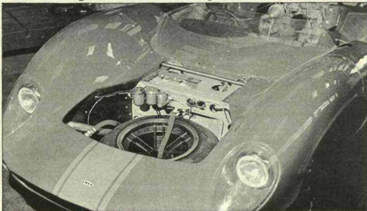
Mk I T70 stowed a spare in the nose; this is Surtees' car at the factory.
