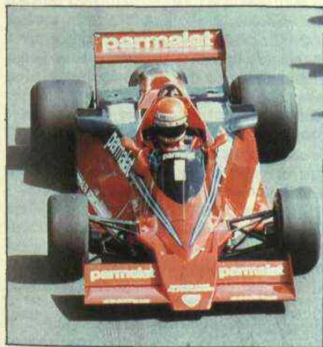
BT46B, the infamous "fan car", won its first and only race in Sweden in 1978, Niki Lauda vanquishing the brilliant Lotus 79. The fan, which created downforce by drawing air from under the car to cool the Alfa engine, was banned as a "moveable aerodynamic device".
