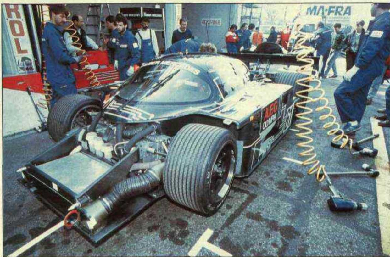
This year's Sauber-Mercedes has improved weight distribution by moving the radiator up to the nose.
