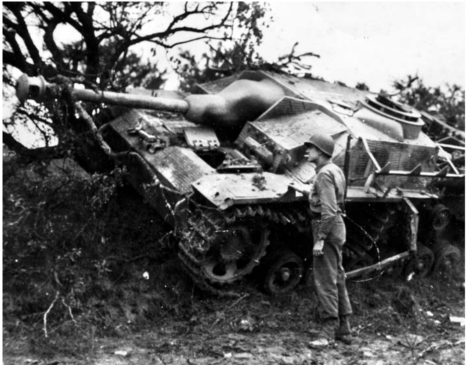
A GI examines a knocked-out Sturmgeschütz III assault gun south of Rechicourt. Such vehicles often replaced the more effective tanks in the depleted German forces in late 1944.
