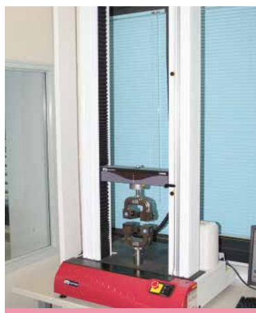
In our Centre for Biotechnological Research "Marco Pozzi", the Shimadzu micro hardness tester and the Instron testing machine are used for the verification of the mechanical properties of the wires.
