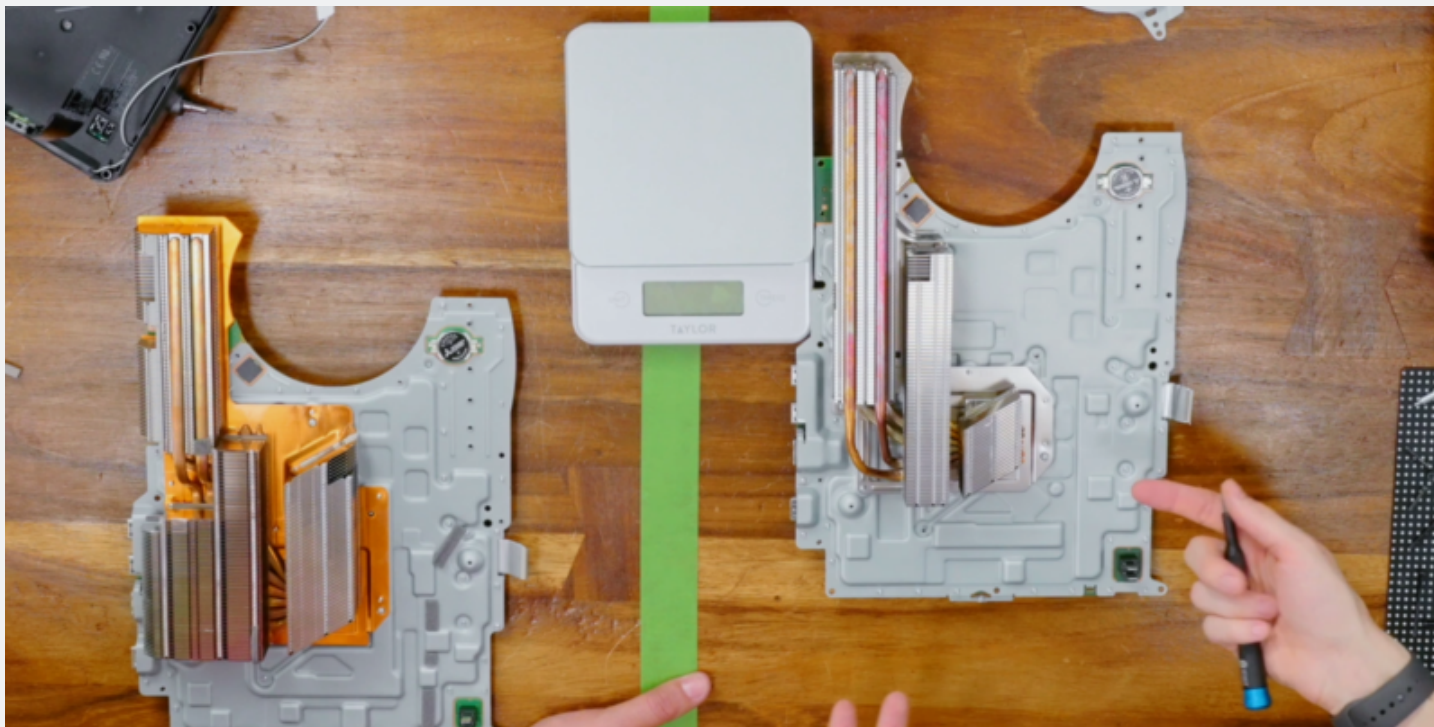
Enlarge / Old PS5 heatsink on the left, new "11-series" PS5 heatsink on the right.
