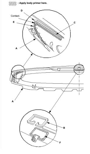
18. Attach the seal (A) with adhesive tape to the upper edge of the extra window (B). Be careful not to touch the windshield where adhesive will be applied.
