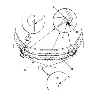
5. Hold a piece of wood, and with a helper on the other side, pull back the piano wire (A) to carefully cut through the adhesive.
