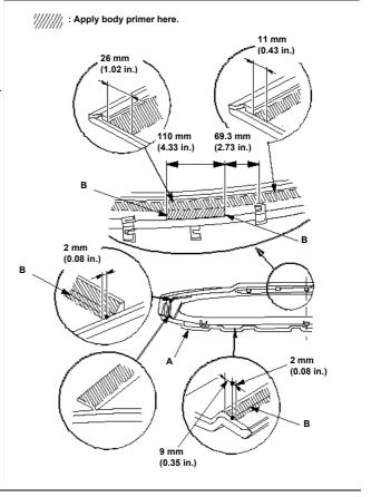
20. With a sponge, apply a light coat of body primer to the original adhesive remaining around the extra window opening flange. Let the body primer dry for at least 10 minutes. Never touch the primed surfaces with your hands.
