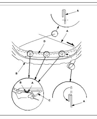
Hold a piece of wood, and with a helper on the other side, pull back the piano wire (A) to carefully cut through the entire extra window adhesive.
